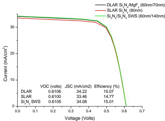
Figure 5. Example I-V curves of solar cells of optimized structures of Si<sub>3</sub>N<sub>4</sub> SWS height of 140 nm and non-etched Si<sub>3</sub>N<sub>4</sub> thickness 60 nm compared with Si<sub>3</sub>N<sub>4</sub> SLAR (80 nm) and Si<sub>3</sub>N<sub>4</sub>/magnesium fluoride DLAR (60 nm / 70 nm) structures obtained from PC1D simulation.
