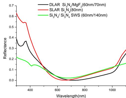
Figure 4. Example Specular optical reflectivity at normal incidence of optimized structures of  $\text{Si}_3\text{N}_4$  SWS height of 140 nm and non-etched silicon nitride thickness 60 nm compared with silicon nitride SLAR (80 nm) and silicon nitride/magnesium fluoride DLAR (60 nm / 70 nm) structures.
