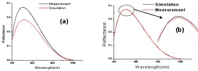
Figure 2. RCWA calculated specular optical reflectivity at normal incidence and measurement reflectivity for  $\text{Si}_3\text{N}_4$  layer of thickness 200 nm deposited on silicon substrate of which 88 nm is the SWS height and 112 nm remained as non-etched. (a) Results with the constant silicon refractive index of 4.35. (b) Results with the silicon refractive index given by a calibrated equation.
