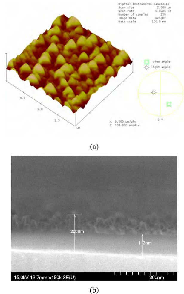
Figure 1. Morphology of the fabricated  $\text{Si}_3\text{N}_4$  SWS (a) AFM Image and (b) SEM Image.
