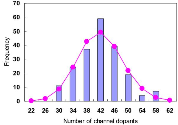
Figure 4. The distribution of the number of channel dopants. The curve is Poisson distribution.
