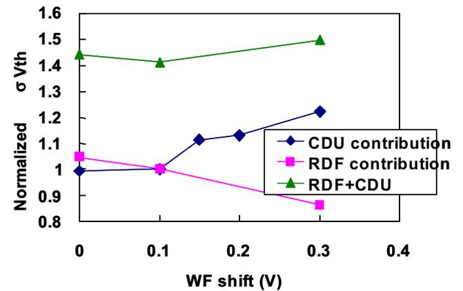
Figure 9. The normalized  $\delta V_{th}$  (RDF, CDU and their total effect) v.s. WFS. A minimum  $\delta V_{th}$  exists with optimum WFS.
