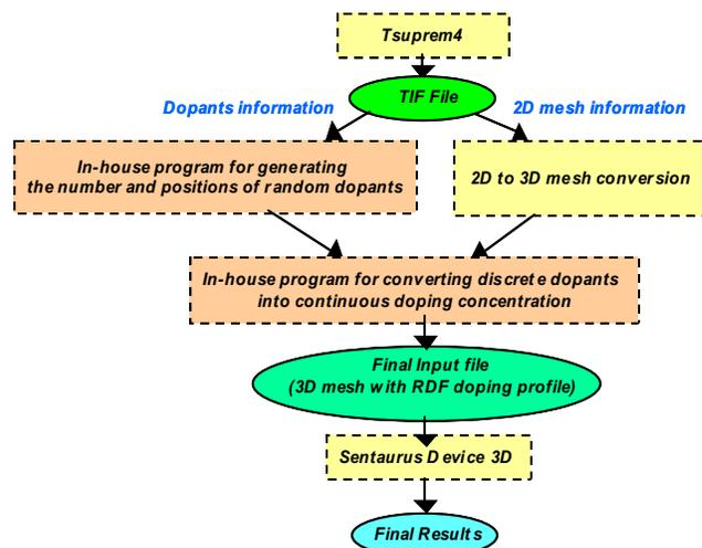
Figure 1. In-house simulation flow for RDF.
