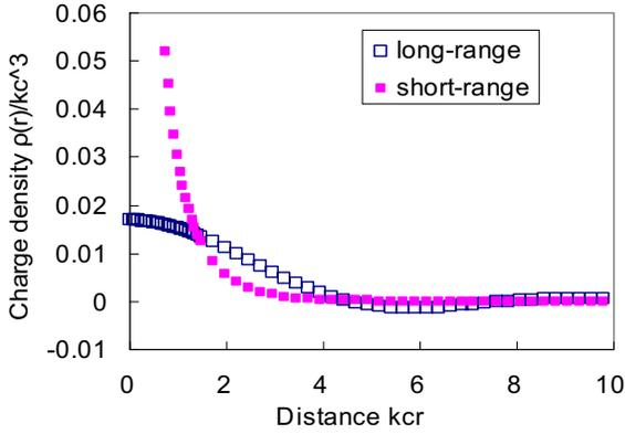
Figure 2. charge density of a single dopant for long-range shown in eq.2 and short-range as a function of distance
