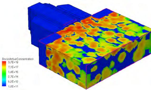
Figure 3. The boron doping profile after considering RDF for further SDevice 3D simulation
