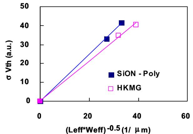
Figure 8. Pelgrom plot of SiON-Poly and HKMG nMOSFETs. The WFS of HKMG nMOSFET is 0.1V and EOT ratio between HKMG and SiON-Poly is about 0.7. The gate dielectric in either case is assumed to be ideal.
