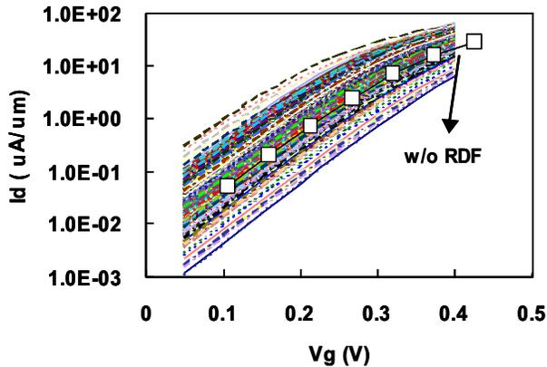
Figure 5. Id-Vg curves of RDF samples. The one without RDF is also shown for comparison.
