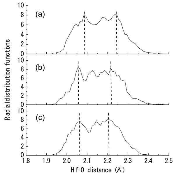
Figure 4. Radial distribution functions of Hf-O in  $\text{HfO}_2$  with (a) 1% strain, (b) no strain and (c) -1% strain along b-axis.
