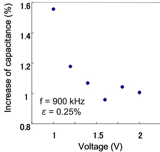
Figure 7. Change of capacitance in MOS capacitor using a HfO<sub>2</sub> gate dielectric by tensile strain.
