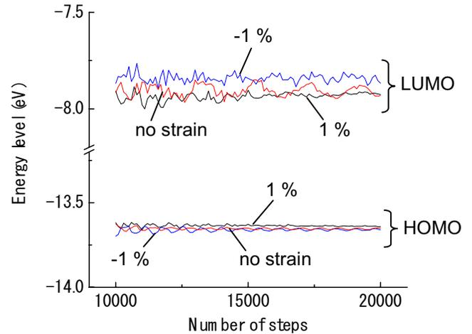
Figure 3. Change in the energy level of HOMO and LUMO in  $\text{HfO}_2$  with 1% and -1% strain along b-axis during simulation.
