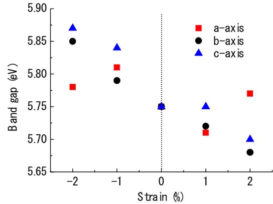
Figure 2. Strain dependence of band gap of monoclinic  $\text{HfO}_2$ .
