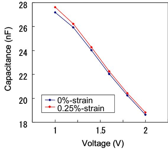
Figure 6. Effect of tensile strain on a capacitance of MOS capacitor using a HfO<sub>2</sub> gate dielectric.
