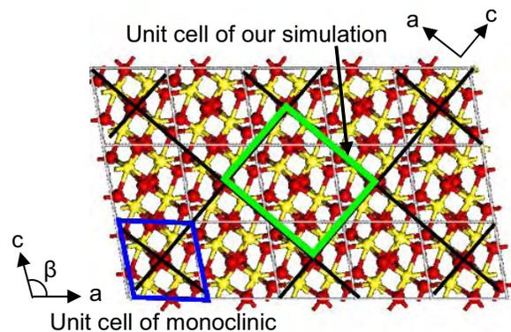
Figure 1. Relationship between the ideal monoclinic structure and our simulation model for  $\text{HfO}_2$  with monoclinic phase.
