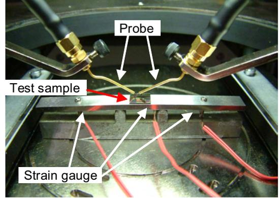
Figure 5. Outlook of four-point bending method.
