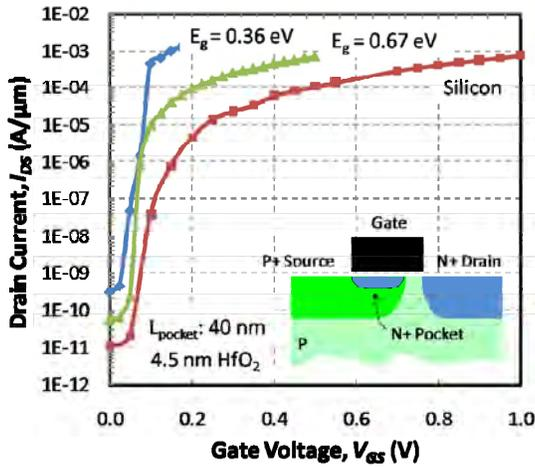
Fig. 8: Reducing  $E_g$  of the tunnel junction allows for supply voltage reduction with large drive current.
