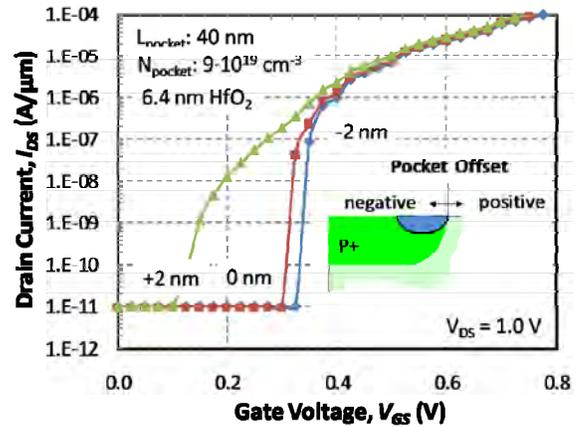
**Fig. 7:** Impact of pocket offset with respect to edge of the source on “turn on” characteristics. Negative offset is defined as the pocket enclosed by the source doping.
