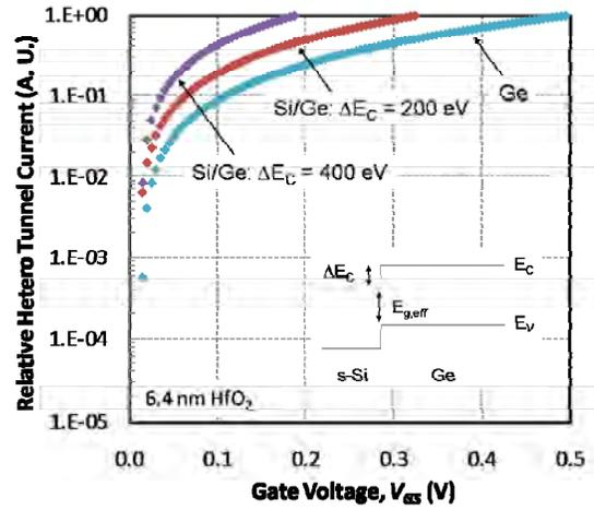
Fig. 10: Relative Si/Ge hetero-tunneling current  $I_D-V_g$  generated from 1D hetero WKB model for various  $E_c$  offsets compared to pure Ge tunnel current. Larger offset or smaller effective band gap allows for smaller gate voltage.
