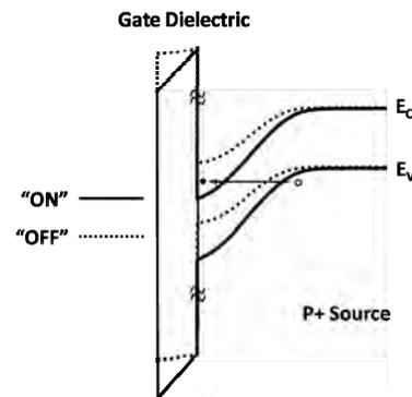
**Fig. 3:** Band diagram of proposed tunnel transistor in “on” and “off” states. No alignment of states in “off” condition.
