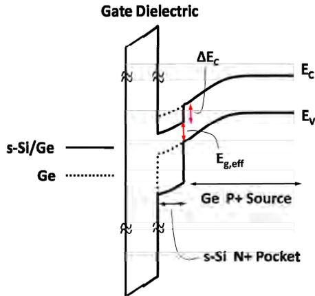
Fig. 9: Large  $E_c$  offset, determined by the amount of strain in Si cap, allows for low effective tunnel band gap.
