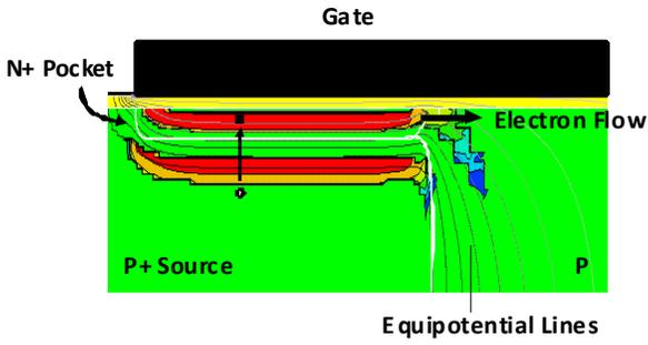
**Fig. 4:** BTBT generation rate contours for proposed tunnel transistor in “on” state. Lower and upper rate contours represent hole and electron generation.
