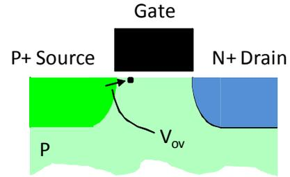
**Fig. 1:** Structure of conventional n-type tunnel transistor. The overlap voltage,  $V_{ov}$ , is the gate voltage at which tunneling occurs when states are aligned.
