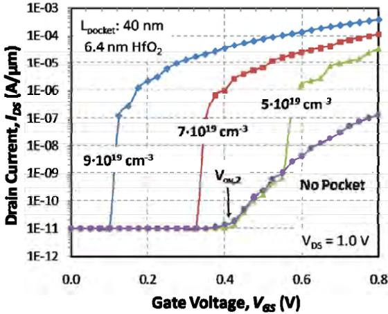
**Fig. 5:** Importance of pocket doping to achieve  $V_{ov,1} < V_{ov,2}$  criteria. Pocket dose lowers overlap voltage  $V_{ov,1}$ .
