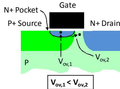
**Fig. 2:** Proposed n-type tunnel transistor with ultra shallow pocket.  $V_{ov,1}$  is the overlap voltage for source/pocket tunneling.  $V_{ov,1}$  must be less than  $V_{ov,2}$  for steep “turn on”.
