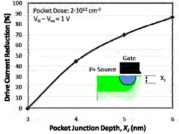
**Fig. 6:** Increased pocket junction depth for fixed dose reduces  $I_{on}$  due to reduced gate capacitive coupling.
