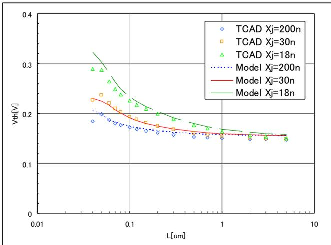
Figure 8: Threshold voltage by TCAD and our model for  $N_c = 5E17 [\text{cm}^{-3}]$ ,  $N_p = 2.5E18 [\text{cm}^{-3}]$ ,  $L_p = 0.02 [\mu\text{m}]$ ,  $X_j = 18, 30, 200 [\text{nm}]$ ,  $V_{ds} = 0.05 [V]$
