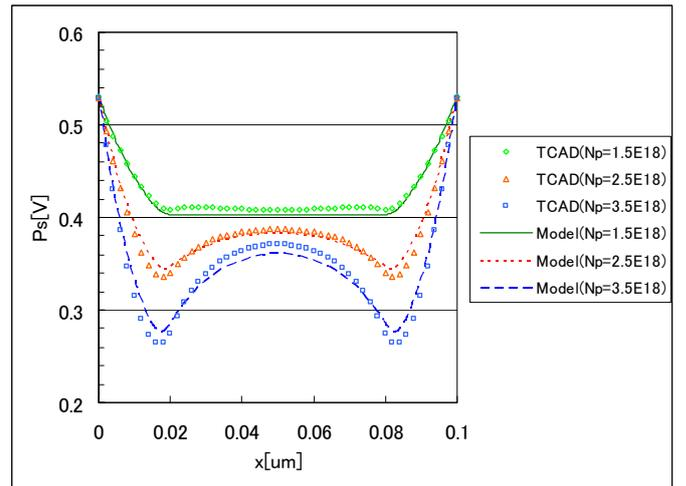
Figure 2: Surface potential by TCAD and our model for  $N_c = 5E17 [cm^{-3}]$ ,  $N_p = 1.5E18, 2.5E18, 3.5E18 [cm^{-3}]$ ,  $L = 0.1 [\mu m]$ ,  $L_p = 0.02 [\mu m]$ ,  $X_j = 30 [nm]$ ,  $V_{ds} = 0 [V]$ ,  $V_{gs} = 0.2 [V]$
