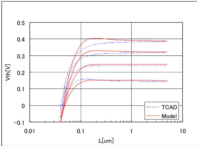
Figure 7: Threshold voltage by TCAD and our model for  $N_c = 5E17 [\text{cm}^{-3}]$ ,  $N_p = 2.5E18 [\text{cm}^{-3}]$ ,  $L_p = 0.02 [\mu\text{m}]$ ,  $X_j = 30 [\text{nm}]$ ,  $V_{bs} = 0, -0.5, -1, -1.5 [V]$ ,  $V_{ds} = 1 [V]$
