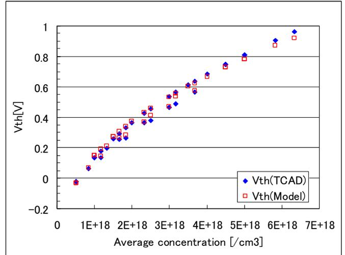
Figure 9: Threshold voltage by TCAD and our model for channel concentration of various combinations of  $N_c, N_p, L_p$ ,  $L = 0.06 [\mu\text{m}]$ ,  $X_j = 18 [\text{nm}]$ ,  $V_{ds} = 0.05 [V]$
