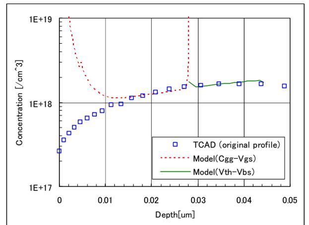
Figure 5: The original profile of TCAD simulation and channel profiles transformed from  $C_{gg} - V_{gs}$  and  $V_{th} - V_{bs}$  by our model for
