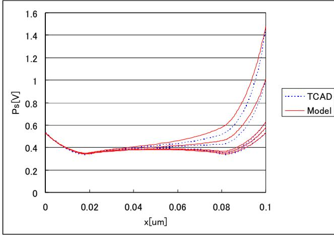
Figure 3: Surface potential by TCAD and our model for  $N_c = 5E17[\text{cm}^{-3}]$ ,  $N_p = 2.5E18[\text{cm}^{-3}]$ ,  $L = 0.1[\mu\text{m}]$ ,  $L_p = 0.02[\mu\text{m}]$ ,  $X_j = 30[\text{nm}]$ ,  $V_{ds} = 0, 0.05, 0.1, 0.5, 1[\text{V}]$ ,  $V_{gs} = 0.2[\text{V}]$
