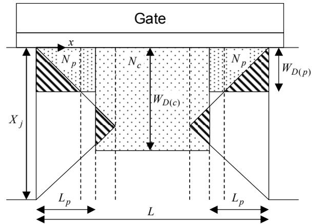
Figure 1: Division of channel region (by dot lines) In regions painted by oblique lines, the charge is ignored when solving Poisson equations.
