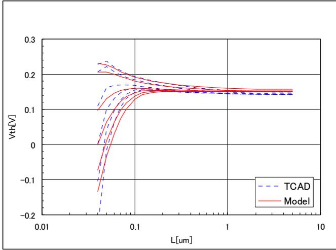
Figure 6: Threshold voltage by TCAD and our model for  $N_c = 5E17 [\text{cm}^{-3}]$ ,  $N_p = 2.5E18 [\text{cm}^{-3}]$ ,  $L_p = 0.02 [\mu\text{m}]$ ,  $X_j = 30 [\text{nm}]$ ,  $V_{ds} = 0, 0.05, 0.1, 0.5, 1 [V]$
