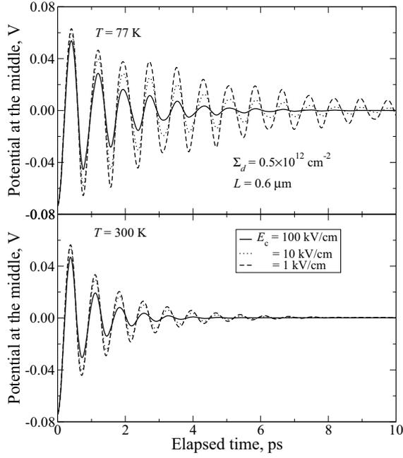
Fig. 3. Potential at  $x = 0$  vs elapsed time for systems with different temperatures and different characteristic electric field  $E_c$ .
