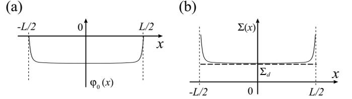
Fig. 2. Schematic views of (a) steady-state potential and (b) steady-state electron concentration in the channel.
