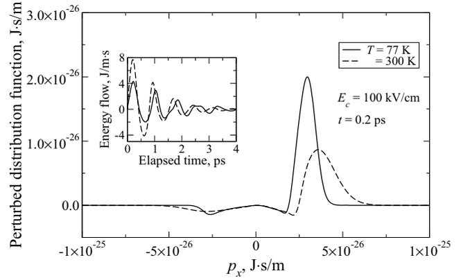
Fig. 5. Perturbed distribution functions at the right contacts,  $(f - f_0)_{x=L/2}$ , at  $t = 0.2$  ps with  $E_c = 100$  kV/cm and different temperatures. The inset shows the evolution of the energy flow at  $x = L/2$ .
