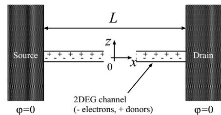
Fig. 1. Geometry of the 2D electron system under consideration.
