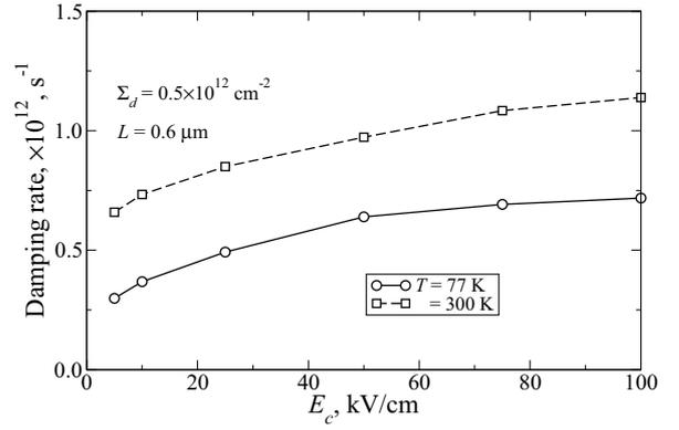
Fig. 4. The damping rate  $\gamma$  as a function of the characteristic electric field  $E_c$ , with different temperature.
