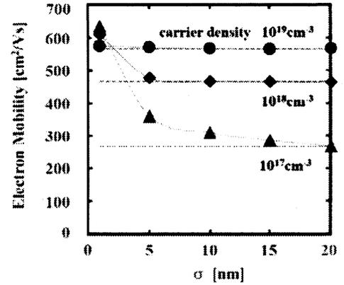
Fig.2 Calculated mobility of electrons as a function of  $\sigma$  of the dopant array. The concentration of the acceptor ions is set to  $10^{18} \text{ cm}^{-3}$ . Dashed lines show the motilities in the randomly distributed dopants.
