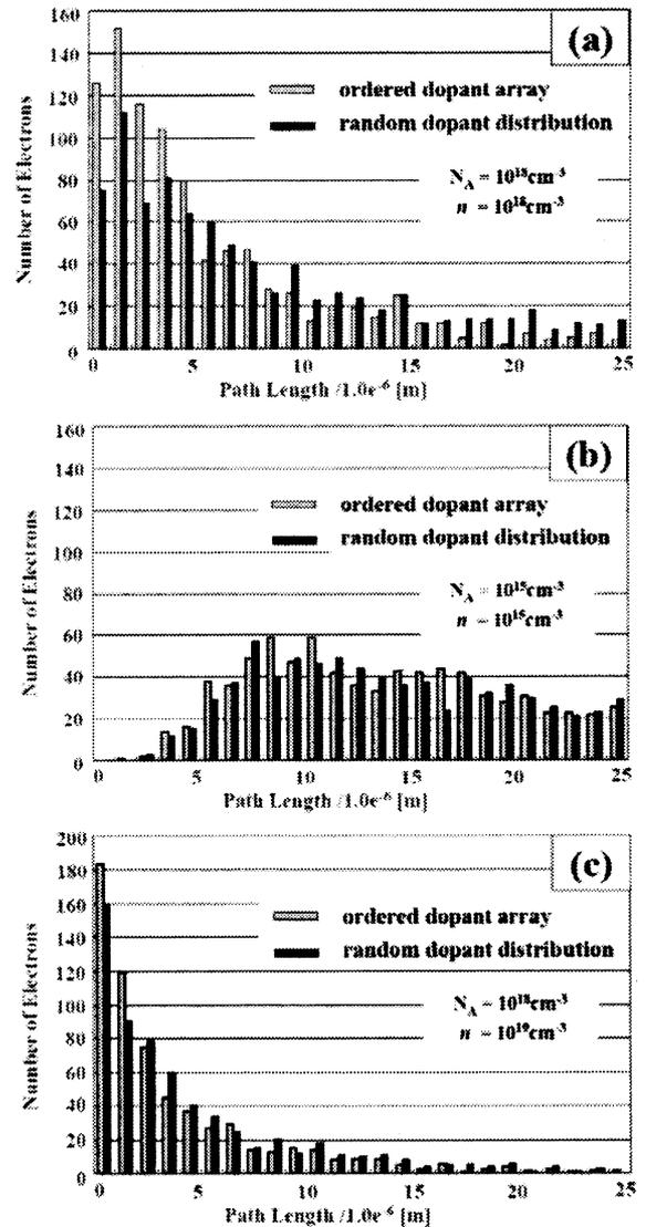
Fig.5 Histogram of the electron path length while the electron goes the distance of  $L (=10^{-7} \text{ m})$  in the direction of the electric field. (a)  $N_A = 10^{18} \text{ cm}^{-3}$ ,  $n = 10^{18} \text{ cm}^{-3}$ , (b)  $N_A = 10^{15} \text{ cm}^{-3}$ ,  $n = 10^{15} \text{ cm}^{-3}$ , and (c)  $N_A = 10^{18} \text{ cm}^{-3}$ ,  $n = 10^{19} \text{ cm}^{-3}$ .
