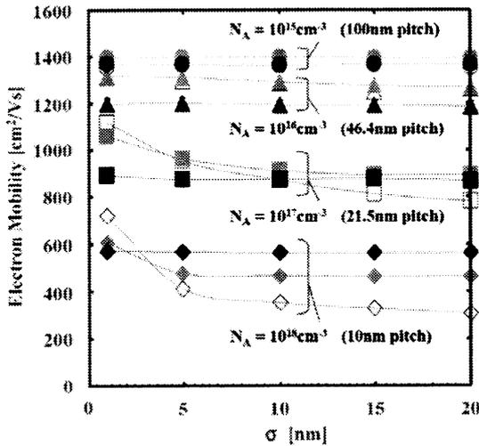
Fig.4 Calculated mobility of electrons as a function of standard deviation  $\sigma$  of the dopant array. The concentration of the acceptor ions is set to  $10^{15} \text{ cm}^{-3}$  (circle marker),  $10^{16} \text{ cm}^{-3}$  (triangle),  $10^{17} \text{ cm}^{-3}$  (square),  $10^{18} \text{ cm}^{-3}$  (diamond). The electron concentration is set to equal (gray), 10 times as much as (solid), one-tenth (open) of the acceptor ions.
