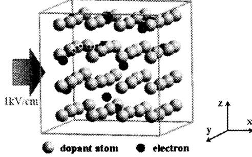
Fig.1 Schematic view of the simulation system for electron transport in Si with ordered dopant array.
