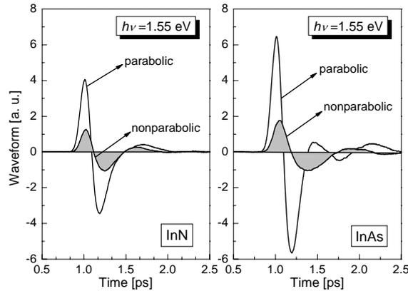
Fig. 3. Temporal THz electric field waveforms for InN (a) and InAs (b) simulated for the laser excitation energy  $h\nu = 1.55$  eV.
