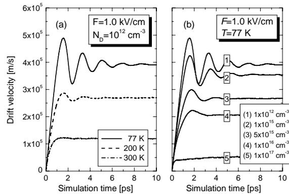
Fig. 1. Transient drift velocity in InN simulated by the EMC method at (a) different temperatures and for (b) different doping levels. The frequency of the damped oscillations is 600 GHz.
