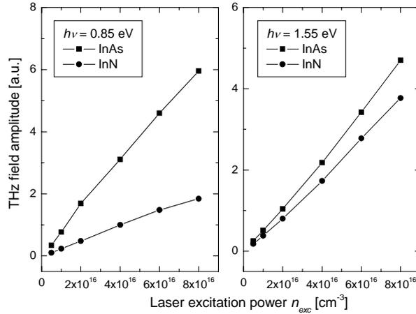
Fig. 5. THz waveform amplitudes for InN and InAs as a function of laser excitation power for photon energies (a)  $h\nu = 0.85 \text{ eV}$  and (b)  $h\nu = 1.55 \text{ eV}$ .
