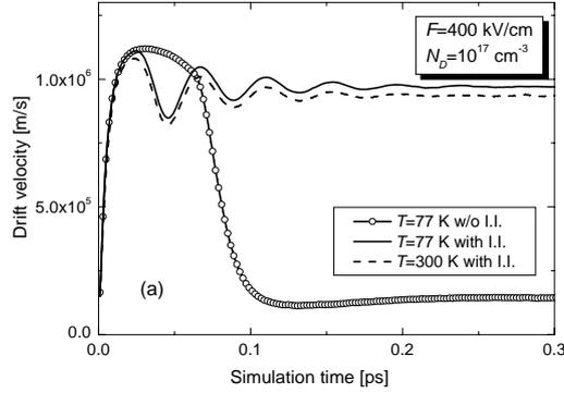
Fig. 2. Transient drift velocity in InN with and without impact ionization simulated by the MC method at different temperatures. The frequency of the damped oscillations is 23 THz.
