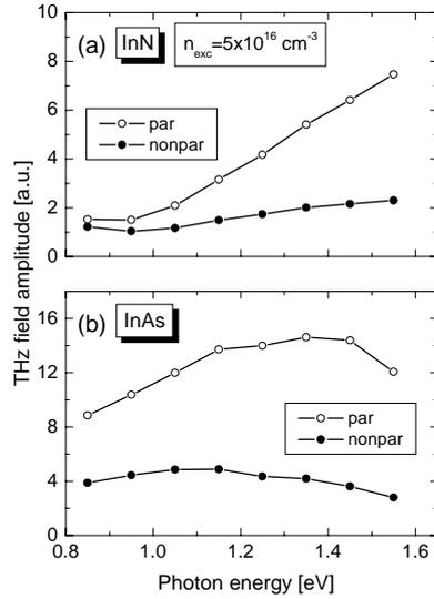
Fig. 4. THz waveform amplitudes for InN (a) and InAs (b) as a function of laser excitation energy.
