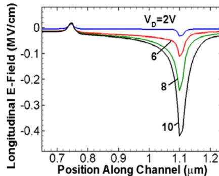
**Figure 8:** Electric field in HD model with AlN IL and  $\tau_e=0.01$  ps in AlGaIn.
