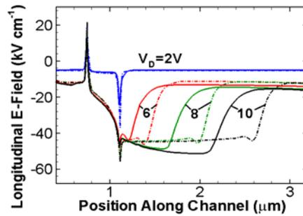
**Figure 4:** Electric field for HD model with (solid) and without (dashed) AlN IL.
