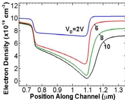
**Figure 7:** Electron density in HD model with AlN IL and  $\tau_e=0.01$  ps in AlGaIn.
