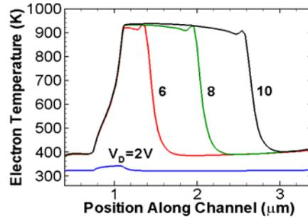
**Figure 2:** Electron temperature for HD model for a HEMT without AlN layer.
