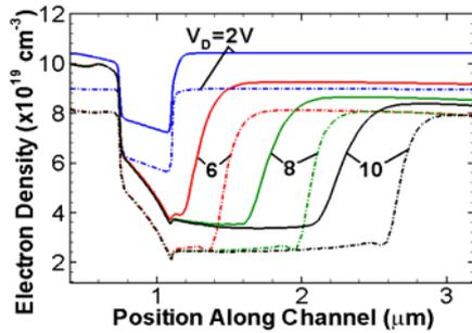
**Figure 1:** Electron density for HD model with (solid) and without (dashed) AlN IL.
