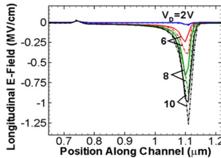
**Figure 6:** Electric field for DD model with (solid) and without (dashed) AlN IL.
