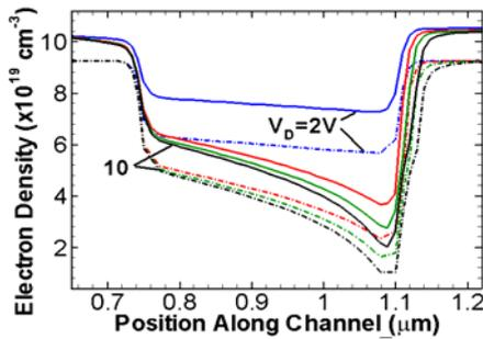
**Figure 5:** Electron density for DD model with (solid) and without (dashed) AlN IL.
