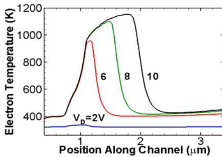
**Figure 3:** Electron temperature for HD model for a HEMT with AlN IL.
