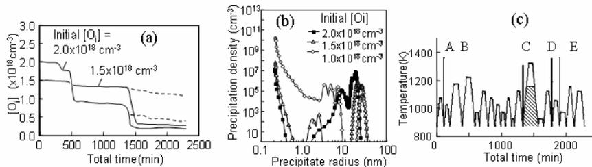
Figure 3: (a) Simulated results of  $[O_i]$  concentration as a function of process sequence for various initial  $[O_i]$  concentrations. (b) Radius distribution of BMD. (c) Typical input process sequence of scaled devices which we have simulated and done on experiments.
