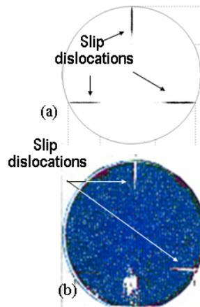
Figure11: (a) Dislocation slip simulation during an RTP. For simplicity, slip lines are modeled to be generated at supporting points and to be moved in stress field. Slip lines grow up until meeting BMD. (b)Experimental result of slip patterns on a wafer.
