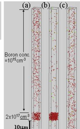
Figure 9: Simulation results of Cu diffusion and gettering characteristics. (a)Initial and (b)60min after at R.T. (c)Snapshot after elevating temperature from R.T. to 200 °C. Cu atoms are captured partly at BMD sites.
