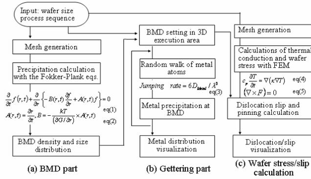
Figure 1: System diagram of wafer processing tool. (a) is a BMD radius,  $f(z,t)$  a size distribution function and  $G$  Gibbs free energy. (b) Metal atoms are treated as particles. (c)  $T$ ,  $\kappa$  and  $F$  are temperature, thermal conductivity and force.
