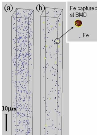
Figure 8: Snapshots of Fe gettering simulation. Fe distributions at  $t=t_1$  and  $t=t_2$  in Fig. 8 are shown in (a) and (b). Execution area is  $10 \times 10 \times 300 \mu\text{m}$ .
