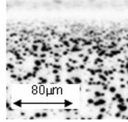
Figure 5: Experimental result of IR tomography. Dots present BMD.
