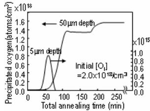
Figure 4: Simulation results of oxygen precipitation for various regions.
