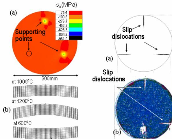
Figure10: Simulation results of (a)stress distribution and (b)distortion for 300mm wafer during typical FLA process.
