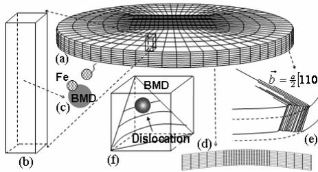
Figure 2: Schematic illustrations of mesh structure, models implemented and execution areas. (a) Wafer mesh, (b) area of BMD execution, (c) gettering model concept, (d) thermal stress calculation, (e) generation of slip, and (f) model for dislocation pinning with BMD.
