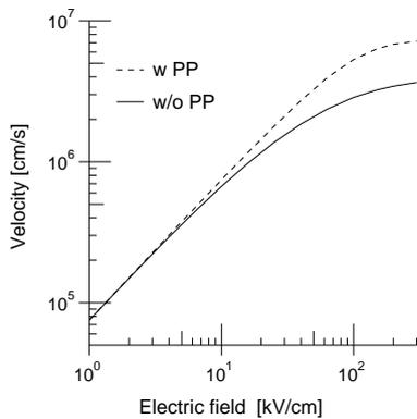
**Figure 3:** Drift velocity calculated with the Pauli principle (w PP) and without (w/o PP) for an electron concentration of  $10^{21}/\text{cm}^3$  in silicon at 300K.
