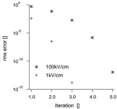
**Figure 1:** Root mean square error of the distribution function for an electron concentration of  $10^{21}/\text{cm}^3$  in silicon at 300K.
