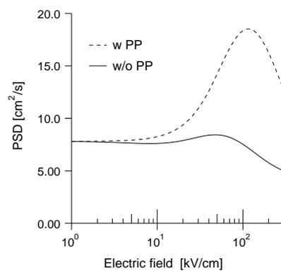
**Figure 4:** Power spectral density of the velocity fluctuations calculated with the Pauli principle (w PP) and without (w/o PP) for an electron concentration of  $10^{21}/\text{cm}^3$  in silicon at 300K.
