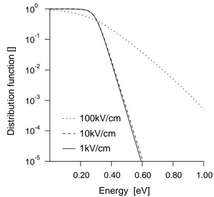
**Figure 2:** Electron distribution function in the valley with the principle axis along the electric field, which is in  $\langle 100 \rangle$  direction, for silicon at 300K.
