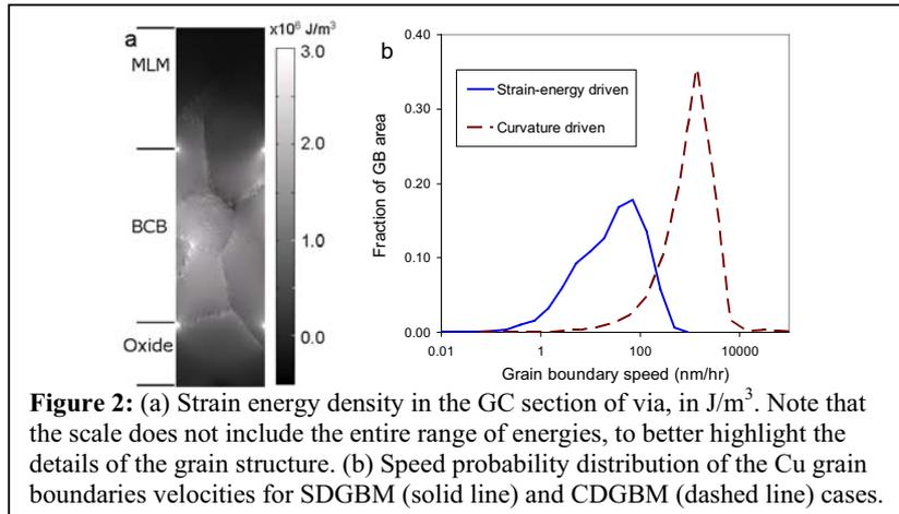
**Figure 2:** (a) Strain energy density in the GC section of via, in  $\text{J/m}^3$ . Note that the scale does not include the entire range of energies, to better highlight the details of the grain structure. (b) Speed probability distribution of the Cu grain boundaries velocities for SDGBM (solid line) and CDGBM (dashed line) cases.
