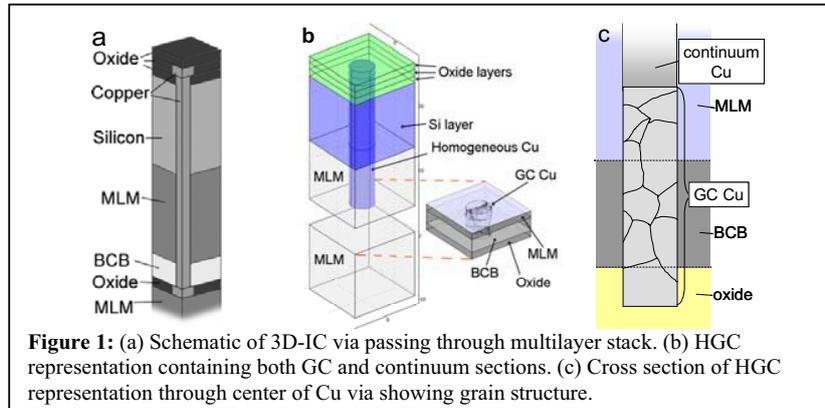
**Figure 1:** (a) Schematic of 3D-IC via passing through multilayer stack. (b) HGC representation containing both GC and continuum sections. (c) Cross section of HGC representation through center of Cu via showing grain structure.
