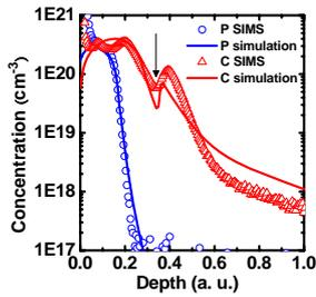
Fig. 2 Comparison of simulated and SIMS profiles of phosphorus diffusion with germanium of 4x energy and carbon coimplants after 1020°C spike anneal. The arrow indicates the position of the a/c interface.
