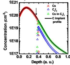
Fig. 1 Simulated as-implanted carbon profile using the modified carbon reactions (1), (2), and (3). The arrow indicates the position of the a/c interface.
