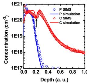
Fig. 3 Comparison of simulated and SIMS profiles of phosphorus diffusion with germanium of 2x energy and carbon coimplants after 1020°C spike anneal. The arrow indicates the position of the a/c interface.
