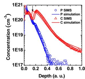
Fig. 4 Comparison of simulated and SIMS profiles of phosphorus diffusion with germanium of 1x energy and carbon coimplants after 1020°C spike anneal. The arrow indicates the position of the a/c interface.
