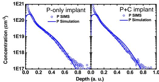
Fig. 5 Comparison of simulated and SIMS profiles of phosphorus-only and phosphorus and carbon coimplant after 1020°C spike anneal.
