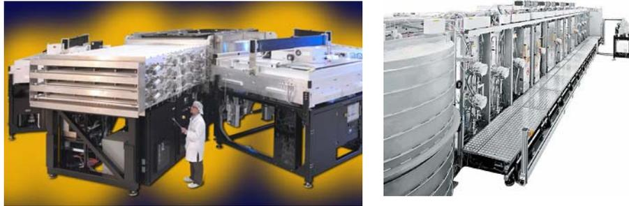
Figure 6 – Large area nanomanufacturing deposition equipment for LCD flat panel displays (a) PECVD cluster tool for the TFT array (b) in-line PVD TCO for color filters.
