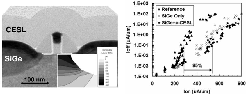
Figure 2 – Strain engineering. (a) TEM of PMOS with SiGe in S/D and c-CESL showing simulated stress contours used to determine local mobilities (b) experimental on-current vs. off-current using different strain enhancement techniques [4].
