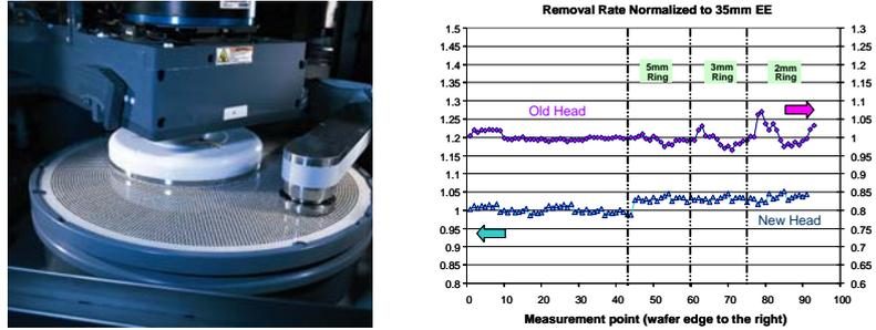
Figure 4 – Chemical mechanical polishing (CMP): (a) Applied Reflexion® LK CMP system and (b) finite element based simulations of CMP material removal rates for two different multizone head designs demonstrating better center to edge uniformity with new design out past the 2mm edge ring for a 300mm wafer [7].
