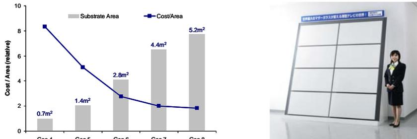
Figure 5 – LCD flat panel production (a) PECVD cost/area reduction with glass size (b) Gen 8 glass substrate used at Sharp Kameyama fab (courtesy Sharp Corporation).
