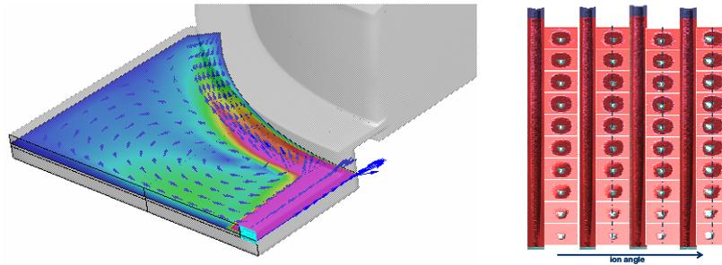
Figure 3 – Examples of equipment simulations where process uniformity is a primary concern (a) flow contours in a 3D epitaxial simulation showing the effect of source gas design [5] and (b) deep trench plasma etch simulations showing the effect of off angle ions on trench shapes towards the edge of a 300mm wafer [6].
