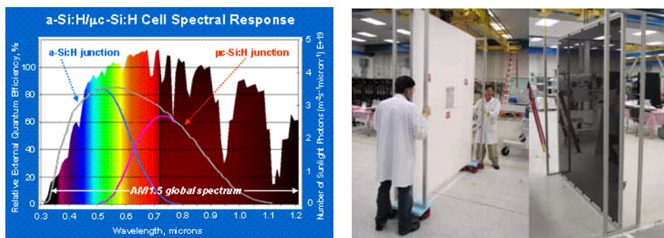
Figure 7 – Thin film silicon solar cells (a) spectral response of a-Si/uc-Si tandem junction (b) Gen 7 panel produced by a large area PECVD tool like that in figure 6a. Note the color of the panel is dark gray indicating the absorber is not pure a-Si.
