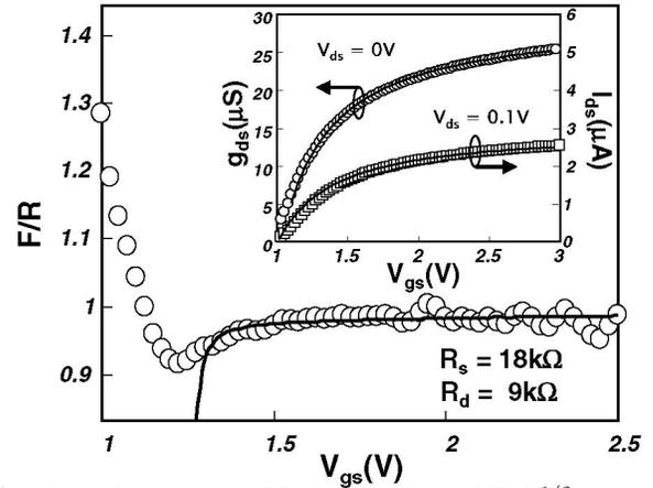
Fig. 3. Forward-reverse ratio of function  $g_{ds}/(dg_{ds}/dV_{gs})^{1/2}$  to detect the asymmetry of the  $R_s$  and  $R_d$ . Open circles are measured data and a solid line is the calculated curve from Eq. 5. Curve fittings using  $g_{ds}$  and  $I_{ds}$  equations with the extracted parameters are in the inset.
