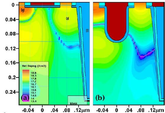
Fig. 7. Cross-section and junction profile obtained from simulation for the asymmetric access transistors: (a) planar, (b) RAD.
