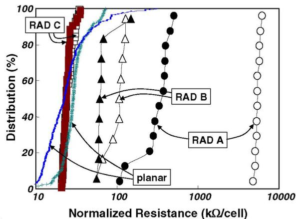
Fig. 9. Distributions of  $R_{ch}$  and  $R_{sd}$  for RAD test structures with different integration processes comparing to the distribution of planar cell transistors from Fig. 4. Solid symbols:  $R_{ch}$ ; open symbols:  $R_{sd}$  distributions.
