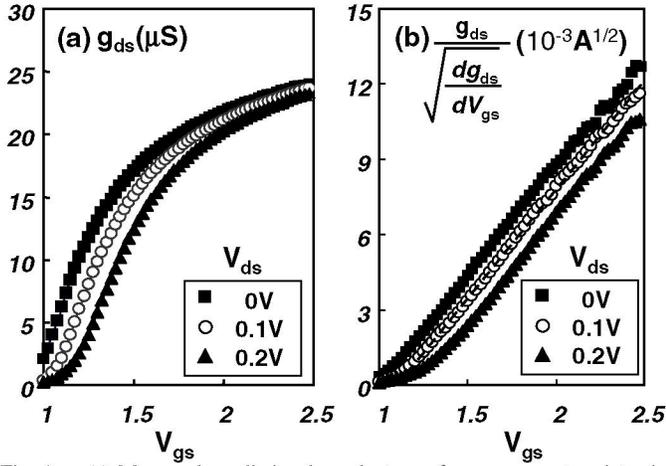
Fig. 2. (a) Measured small-signal conductance for an access transistor in a 78nm technology DRAM cell. (b)  $g_{ds}/(dg_{ds}/dV_{gs})^{1/2}$  curves for a zero drain voltage and two non-zero  $V_{ds}$
