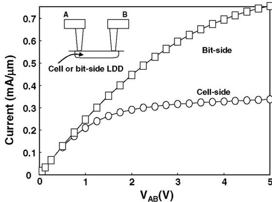
Fig. 5. Simulated  $I$ - $V$  curves for cell and bit-side LDDs and contacts.
