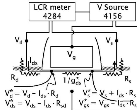
Fig. 1. Schematic of an asymmetric-access transistor of a DRAM cell and the definition of variables, including series resistances and internal and external (applied) voltages on the transistor.
