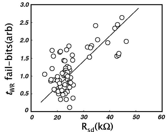
Fig. 6. Correlation between  $R_{sd}$  and  $t_{WR}$  failure under a specific  $t_{WR}$  sorting condition.
