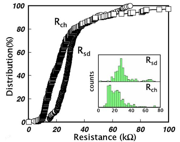
Fig. 4. Distributions of extracted  $R_{sd}$  and  $R_{ch}$ . Differential distributions were depicted in the inset.
