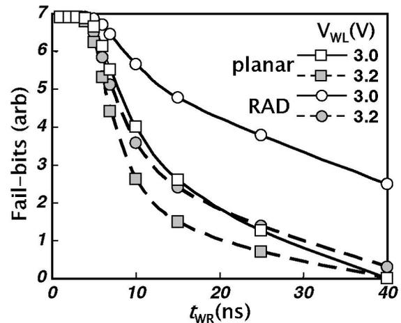
Fig. 8. Fail-bit versus  $t_{WR}$  trends as a function of word-line drive voltage for the DRAM cells with RAD and planar access transistors.
