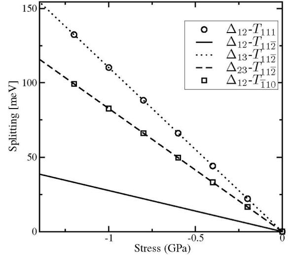
Figure 2: Effect of uniaxial stress on valley splitting ( $\Delta_{ij} = \Delta\epsilon_C^{(j)} - \Delta\epsilon_C^{(i)}$ ) for stress ( $T$ ) along  $[111]$ ,  $[11\bar{2}]$  and  $[\bar{1}10]$  directions.  $T_{hkl}$  denotes the direction of the applied stress.
