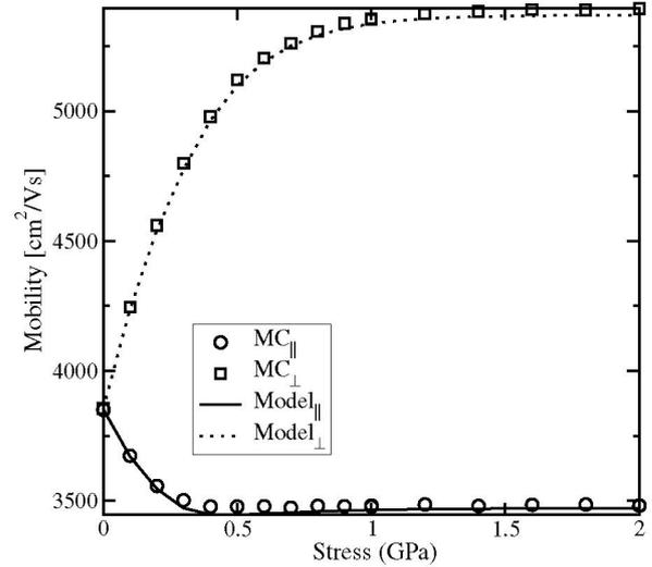
Figure 5: Electron mobility in (111) plane versus uniaxial tensile (along  $[111]$ ) stress at room temperature.  $MC_{||}$  indicates the isotropic in-plane mobility, while  $MC_{\perp}$  denotes the out-of-plane mobility.
