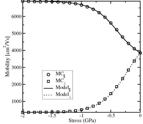
Figure 4: Electron mobility components in (111) plane versus uniaxial compressively (along  $[111]$ ) stress at room temperature.  $MC_{||}$  indicates the isotropic in-plane mobility, while  $MC_{\perp}$  denotes the out-of-plane mobility.
