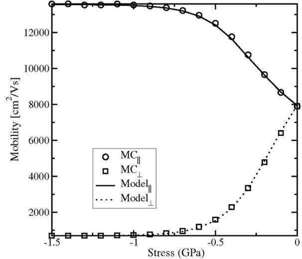
Figure 7: Electron mobility in the (111) plane versus uniaxial compressive stress along [111] at 200K.  $MC_{||}$  indicates the isotropic in-plane mobility, while  $MC_{\perp}$  denotes the out-of-plane mobility.
