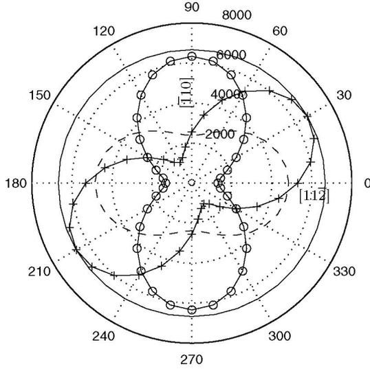
Figure 3: Variation of electron mobility in the (111) plane with the in-plane angle for -1 GPa stress along different directions, at room temperature. Stress directions are represented as:  $[111]$  (solid),  $[11\bar{2}]$  (solid circle),  $[\bar{1}10]$  (dashed) and  $[\bar{1}11]$  (solid +).
