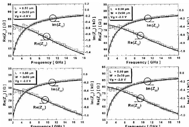
Figure 16. Measured (symbol) and simulated (solid line)  $Z$ -parameters at  $V_g = -2.0 \text{ V}$ .
