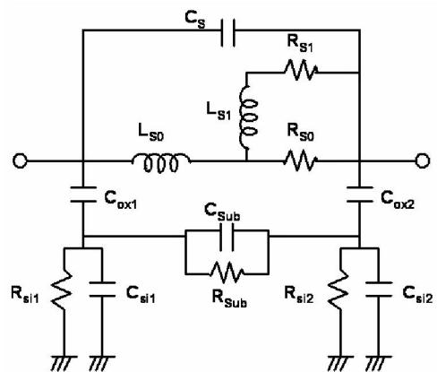
Figure 11. Inductor model with  $R_{sub}$  and  $C_{sub}$  to model substrate effects.
