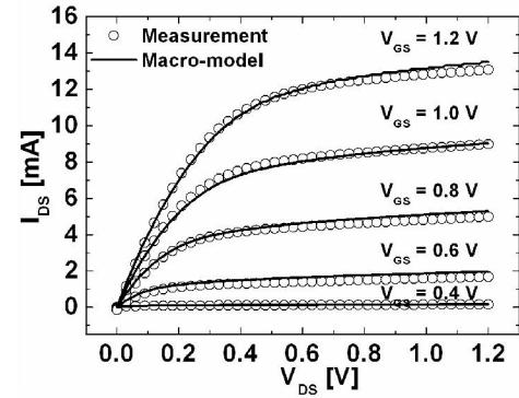
Figure 7. DC  $I_{DS}$ - $V_{DS}$  measurement and simulation data of macro-model.
