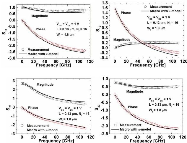
Figure 6. The macro-modeled and measured S-parameters at  $V_{GS} = V_{DS} = 1$  V for 0.13  $\mu\text{m}$  RF nMOSFET ( $T = 125^\circ\text{C}$ ).
