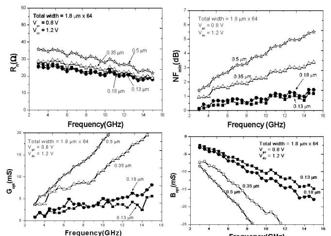
Figure 8. Measured noise parameters of MOSFETs with different channel lengths.
