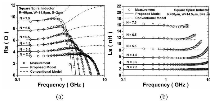
Figure 12. (a) series resistance and (b) series inductance comparison between the measurement and the model.
