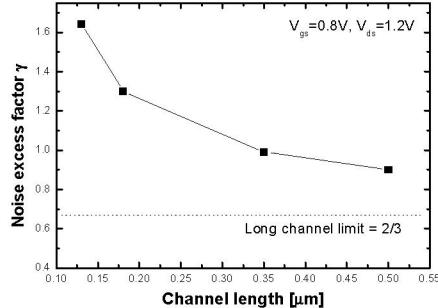
Figure 9. The modeled noise excess factor  $\gamma$  versus channel length for NMOS with fixed  $W = 1.8 \mu\text{m} \times 64$ .
