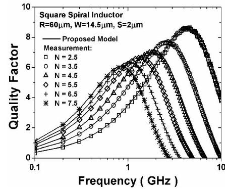
Figure 13. Measured and modeled quality factor of various number of turns.
