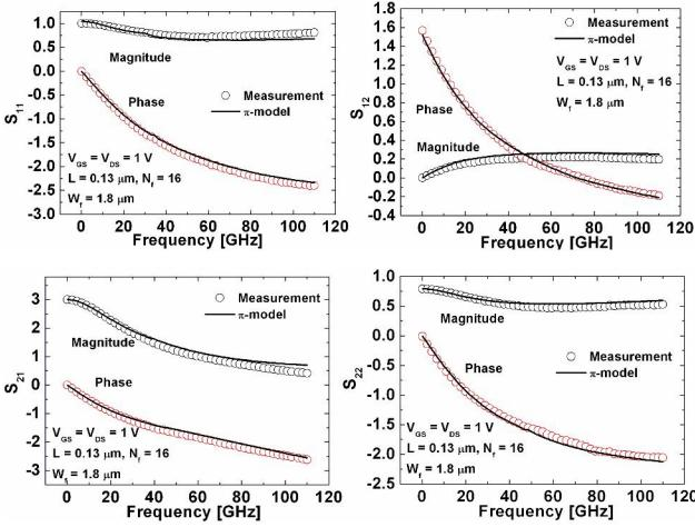
Figure 5. The macro-modeled and measured S-parameters at  $V_{GS} = V_{DS} = 1$  V for 0.13  $\mu\text{m}$  RF nMOSFET ( $T = 25^\circ\text{C}$ ).
