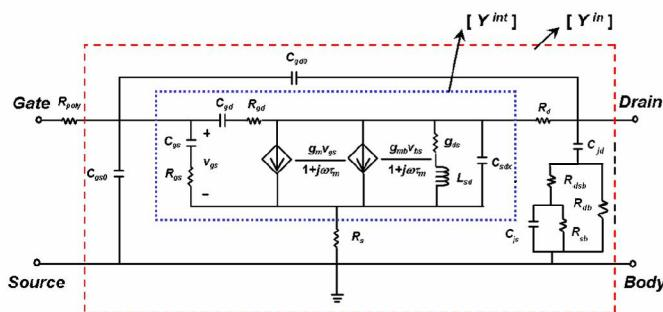
Figure 2. NQS model of RF MOSFET operating in strong inversion region.
