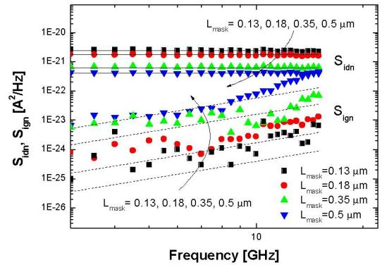
Figure 10. Extracted and modeled channel thermal noise( $S_{idn}$ ) and induced gate noise( $S_{ign}$ ) versus frequency characteristics for n-type MOSFETs biased at  $V_{GS}=0.8V$ , and  $V_{DS}=1.2V$ .
