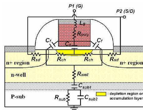
Figure 14. The cross-section of an accumulation-mode MOS varactor.
