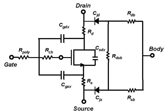
Figure 4. The macro-model for RF MOSFETs, which is implemented as a subcircuit extension to the BSIM4.
