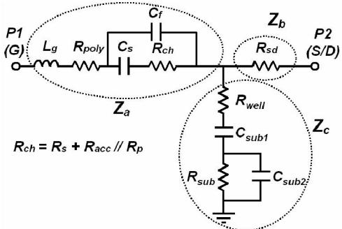
Figure 15. An equivalent circuit for MOS varactor.
