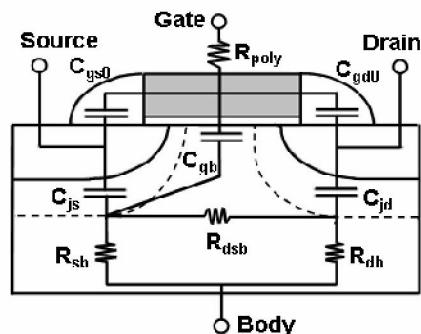
Figure 1. Equivalent circuit of an off-state MOSFET with  $\pi$ -type substrate resistance model.
