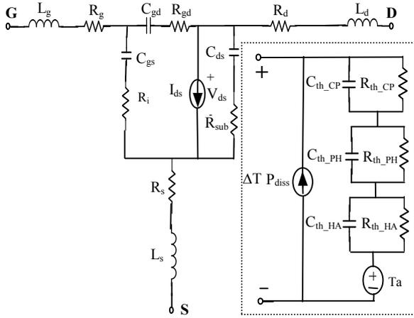
Fig. 2. Large-signal equivalent circuit of the power RF LDMOS model with a thermal circuit including three cells.
