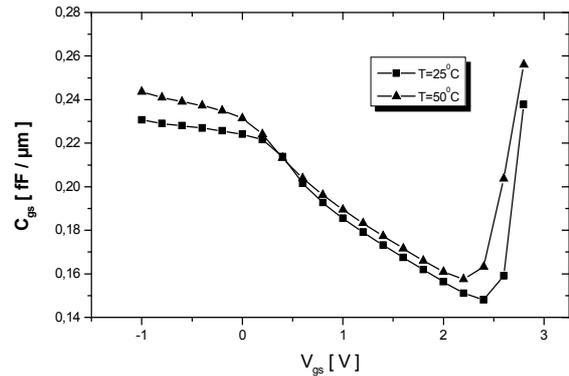
Fig. 10.  $C_{gs}$  obtained from the physical simulation approach (Atlas 2-D) at different  $T_a$ , with Freq=1Mhz
