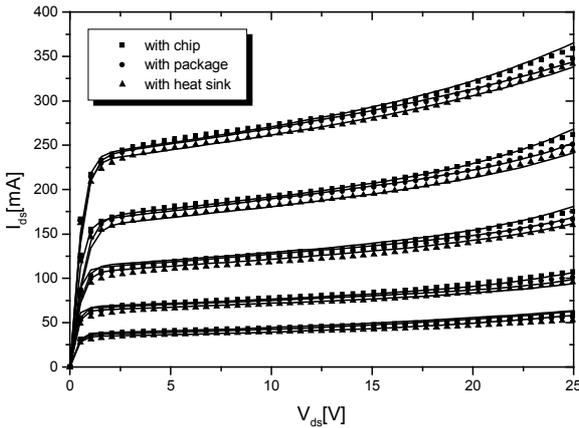
Fig. 3. Measured (dashed) and modeled (line) output characteristic at various conditions,  $V_{gs}=[3 : 6V]$ , step=600mV.
