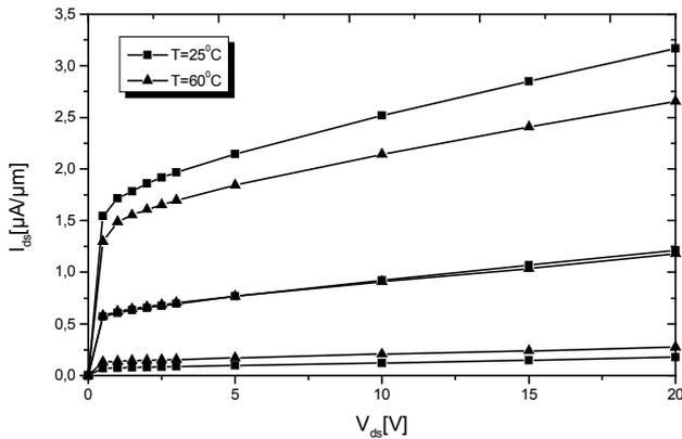
Fig. 6. Output characteristic obtained from a numerical simulation (Silvaco-Atlas) at different  $T_a$ :  $V_{gs} = [1:5V]$ .
