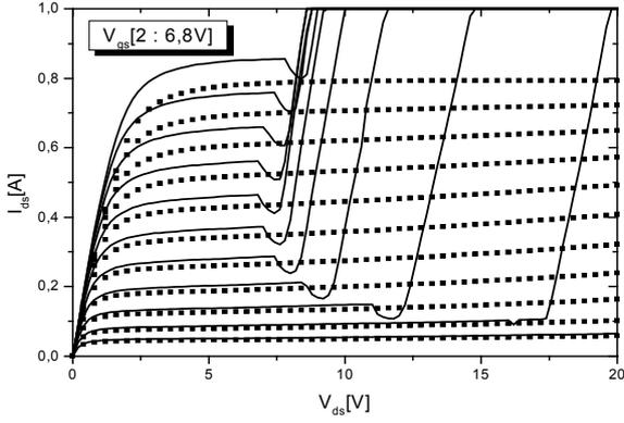
Fig. 1. Output characteristics: Thermal instability effect (line) and stable temperature conditions (dashed).
