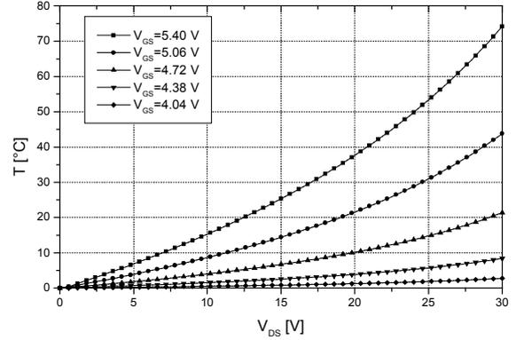
Fig. 4. ADS simulation of the temperature inside the chip, for DC biased condition.
