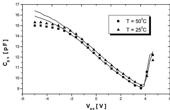
Fig. 8. Measured (dashed) and modelled (line) gate-source capacitance at different  $T_a$ , with Freq=1Mhz
