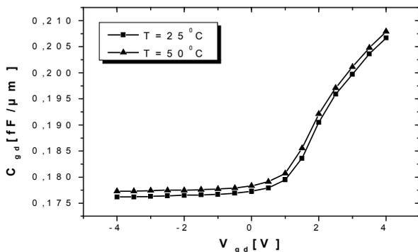
Fig. 9.  $C_{gd}$  obtained from the physical simulation approach (Atlas 2-D) at different  $T_a$ , with Freq=1Mhz
