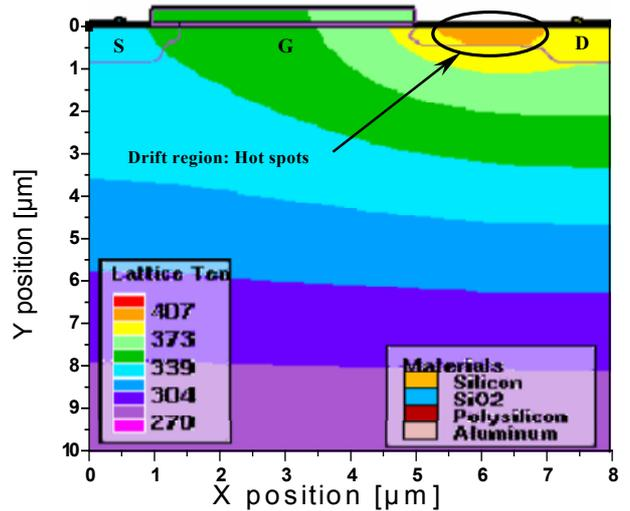
Fig. 5. Distribution of power dissipation and temperature rise within the RF LDMOS at  $T_a: V_{gs} = 8V, V_{ds} = 30V$ .
