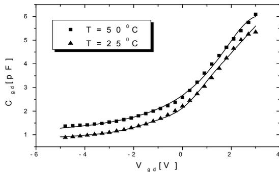
Fig. 7. Measured (dashed) and modeled (line) gate-drain capacitance at different  $T_a$ , with Freq=1Mhz
