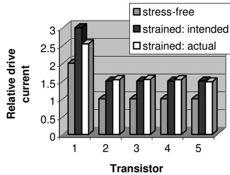
Figure 8: Comparison of the intended relative transistor strength and the actual transistor strength including the non-uniform stress distribution.
