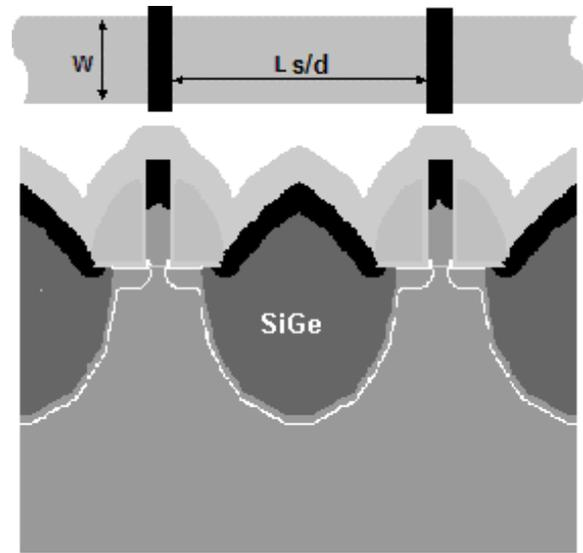
Figure 2: Simulated 2D cross-section of a nest 35nm PMOS. Layout is shown on the top insert.
