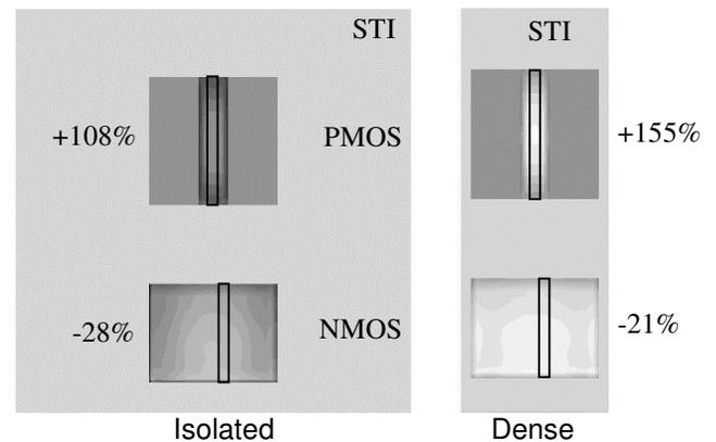
Figure 10: Mobility variation across silicon for NMOS and PMOS transistors in inverters placed in isolated and dense environments. Gate locations are outlined. Also marked is the average low-field mobility stress-enhancement of each transistor.
