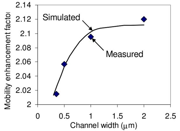
Figure 6: Mobility gain of isolated transistors as a function of channel width. Measured data is shown as symbols, and simulation results are shown as lines.
