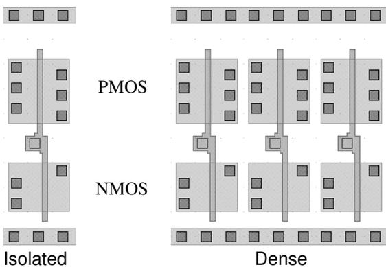
Figure 9: Layout for inverters in isolated and dense environments.
