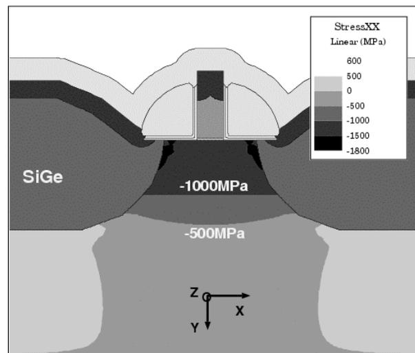
Figure 4: Simulated stress distribution of the normal stress component along the channel direction for a nested PMOS transistor with  $0.4\ \mu\text{m}$   $L_s/d$ .
