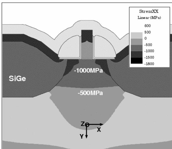
Figure 3: Simulated stress distribution of the normal stress component along the channel direction for an isolated PMOS transistor with  $0.4\ \mu\text{m}$   $L_s/d$ .
