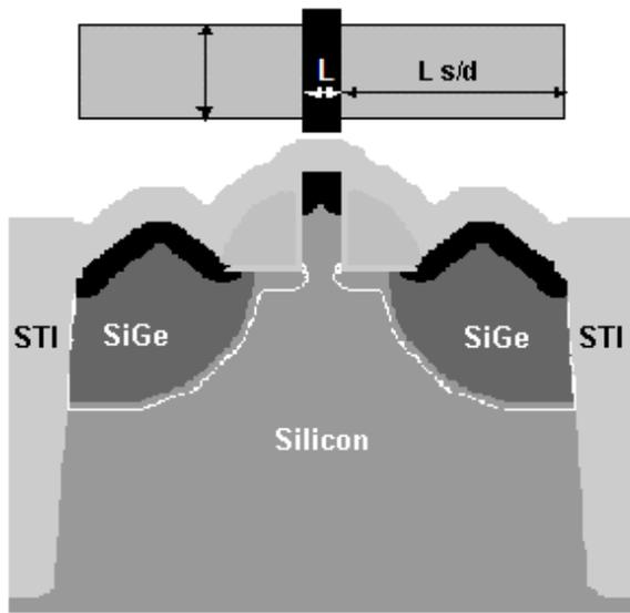
Figure 1: Simulated 2D cross-section of an isolated 35nm PMOS. Layout is shown on the top insert.
