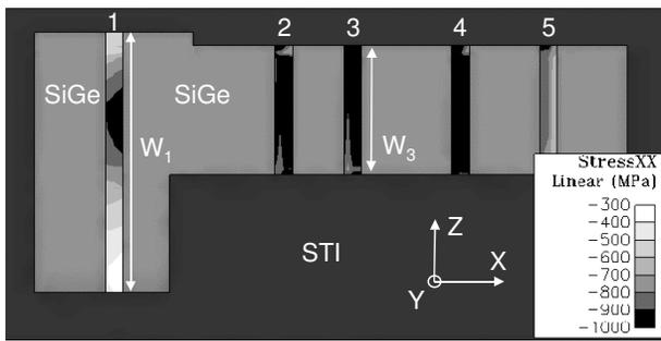
Figure 7: PMOS transistors from a library cell for the 45 nm technology node. Transistor #1 is supposed to have drain current twice as big as the other transistors. Simulated longitudinal stress distribution is shown as a top view of the 3D simulation domain.
