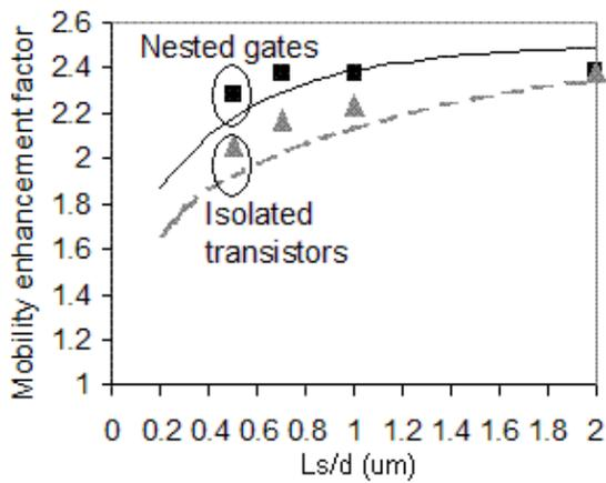
Figure 5: Mobility gain of isolated transistors and transistors with nested gates as a function of  $L_s/d$ . Measured data is shown as symbols and simulation results are shown as lines.
