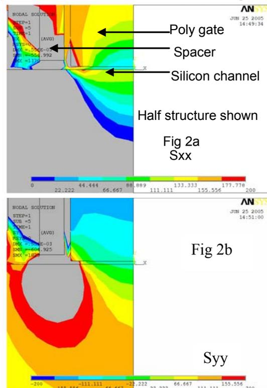
Fig 2: (a) Lateral tensile stress ( $S_{xx}$ ) and (b) Vertical compressive stress ( $S_{yy}$ ) before the ramp to high temperature. Gray areas represent stress values outside of plotted range.
