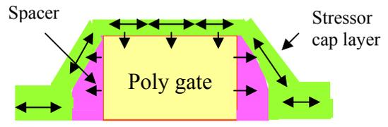
Fig 1: Schematic of the stress “memorization” process. The stressor nitride cap layer is removed subsequent to the source drain anneal.
