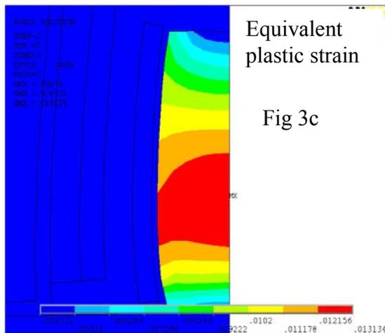
Fig 3a-c: Lateral tensile stress ( $S_{xx}$ ), vertical compressive stress ( $S_{yy}$ ) and equivalent plastic strain at peak temperature. Gray areas represent stress values outside of plotted range. In 3c, the deformation is intentionally exaggerated 15X to show lateral expansion and vertical compression of the poly.
