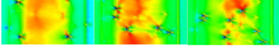
Fig.4: Channel velocity for 3 atomistic MOSFETs with: (left) low, (middle) average and (right) high threshold voltage (blue=low velocity; red=high velocity).
