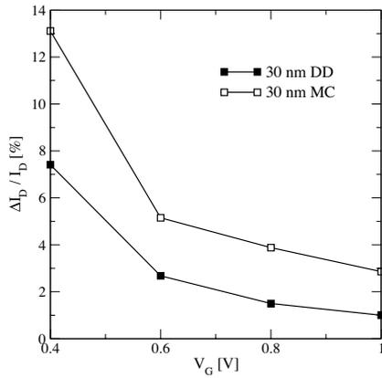
*Fig.2:* Percentage reduction in drive-current upon introducing a trapped charge in the centre of the channel.
