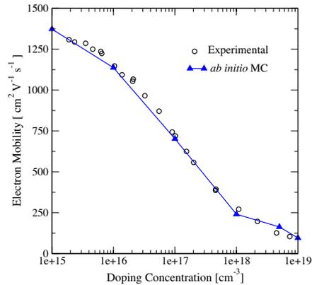
Fig.1: Concentration dependent mobility results using *ab initio* and impurity scattering rates Monte Carlo simulations compared with experimental values.
