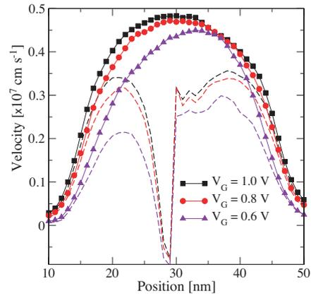
*Fig.3:* Velocity profile through position of trapped charge, placed at 30 nm, with and without the charge present for different gate voltages.
