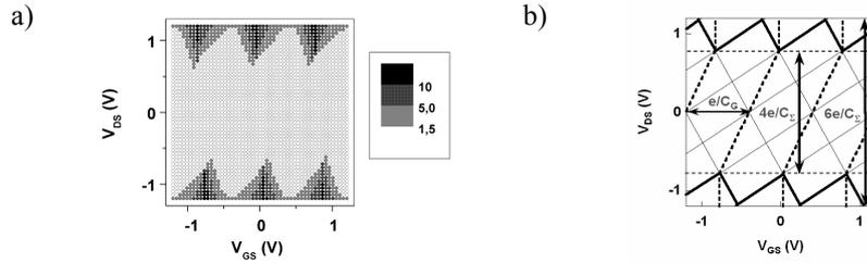
Figure 2: a) Example of relative error (%) between MC simulation and our model in the  $V_{DS}$ - $V_{GS}$  diagram. In the central region the accuracy is better than 1.5%. b) Theoretical limits of validity of our model (which correspond to the MC results).
