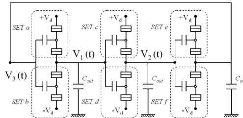
Figure 3: Ring oscillator with 3 SET inverters.
