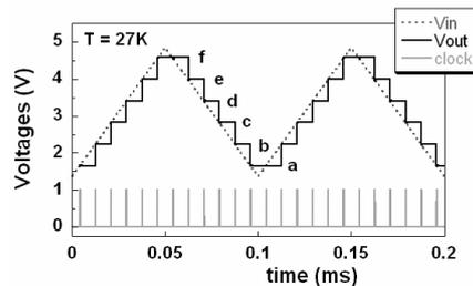
Figure 7: Simulation of the quantizer operation. The output voltage  $V_{\text{out}}$  (with a staircase shape with respect to the stability points) corresponds to the sampling of the triangular voltage  $V_{\text{in}}$ .
