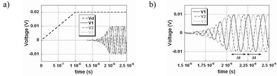
Figure 4: Simulation of the ring oscillator behaviour. When the supply voltage  $V_d$  is increased to its nominal value, the outputs voltages  $V_i$  oscillate (b : zoom of Figure a).
