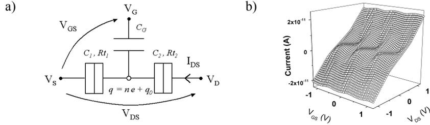
Figure 1: a) Schematic representation of a Single-Electron Transistor. b) Example of current  $I_{DS}$  calculated with our model. The blockade regions (diamond shape) can be clearly distinguished.
