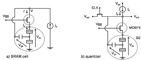
Figure 5: Schematic circuits proposed by Inokawa a) SRAM cell [5] (the multiple-value memory effect is due to the V-I hysteresis). b) "quantizer" [6] (the signal  $V_{in}$  is sampled with respect to the frequency defined by the "Clock" MOSFET along the stability points a, b, ..., f).
