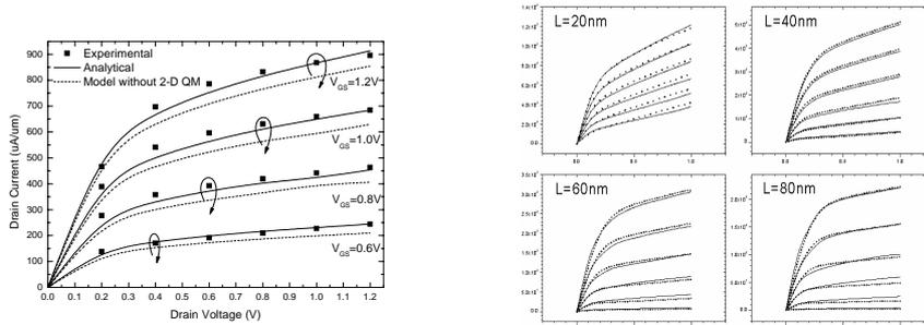
Figure 3 : (a) Output characteristics of the 45nm n-MOSFET from TSMC [1]. (b) Test of scalability. Dash lines are numerical results and solid lines are from BMM.
