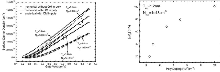
Figure 2 : (a) Surface carrier density with different  $N_p$  and  $T_{ox}$ .  $N_{sub} = 1e18cm^{-3}$ . (b)  $\Delta V_{th,PGqm}$  versus poly-gate doping.
