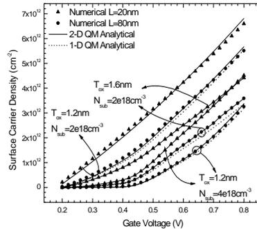
Figure 1 : (a)  $\Delta V_{th,2Dqm}$  vs.  $L$  at  $V_{DS} = 0$ . (b) Surface carrier density vs.  $V_{GS}$ .
