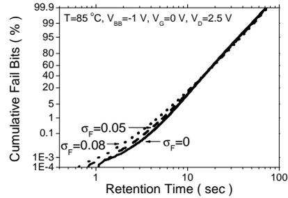
Figure 6: Effect of field fluctuation on the retention time distribution.
