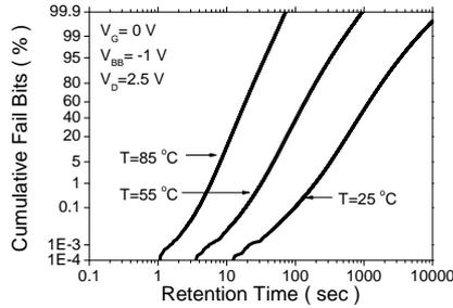
Figure 5: Temperature dependences of the retention time distribution.
