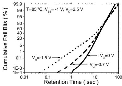
Figure 7: Gate bias dependence of the retention time distribution.
