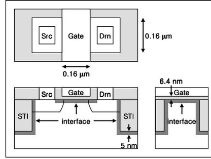
Figure 2: Structure of the DRAM cell transistor.
