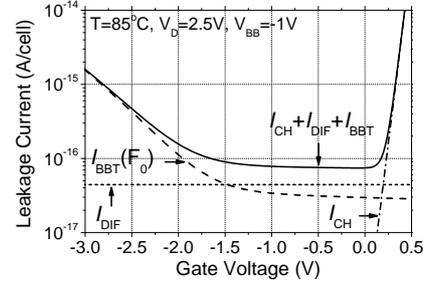
Figure 4:  $I_{\text{DIF}}$ ,  $I_{\text{CH}}$ , and  $I_{\text{BBT}} (F_0)$  vs. gate voltage.
