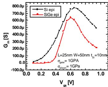
Fig.11: Si and SiGe epi for 25nm SSDOI devices.
