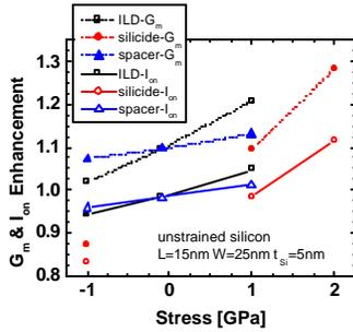
Fig.8:  $I_{on}$  and  $G_m$  enhancements for different stress in ILD, spacer, and silicide.
