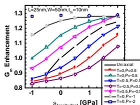
Fig.2:  $G_m$  enhancement for uniformly strained devices in transverse and perpendicular directions.
