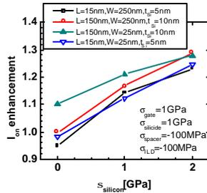
Fig.5: Drive current enhancement for different silicon stress.
