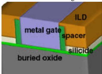
Fig.1: Structure of the ultra thin body device.
