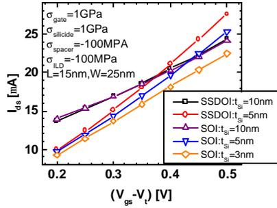
Fig.7:  $I_{ds}$  for a 15nm device with different silicon channel thickness.
