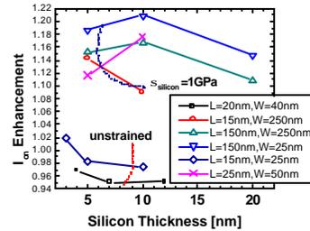
Fig.6: Silicon thickness effect on drive current enhancement.
