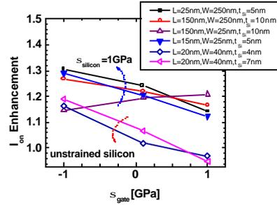
Fig.4: Drive current enhancement for different intrinsic gate stress.
