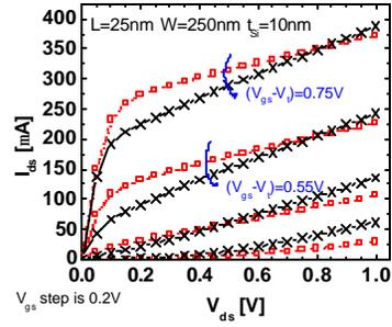
Fig.9: I-V curves for optimal process-induced stress in SSDOI (cross) and SOI (square).
