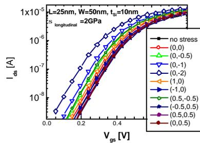
Fig.3: I-V curves for different uniformly strained devices (first number-transverse, second number-perpendicular, in GPa).
