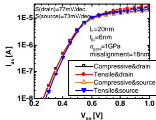
Fig. 11: Transfer characteristics for  $V_{ds}=50mV$  for devices misaligned by 18nm with compressive and tensile metal gates.
