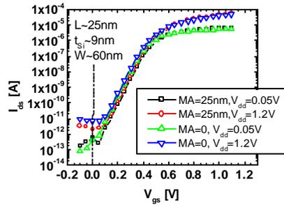
Fig.3: Experimental transfer characteristics for  $L=25\text{nm}$  narrow devices with deliberate gate misalignment of  $25\text{nm}$  toward the drain.
