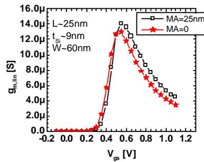
Fig.4: Measured  $g_{m,\text{lin}}$  for  $25\text{nm}$  narrow devices with deliberate gate misalignment.
