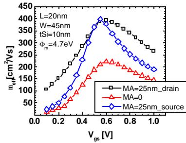
Fig.7: Effective mobility, extracted from simulated data for misaligned 45nm wide transistor ( $L_{eff}=20nm$ ).
