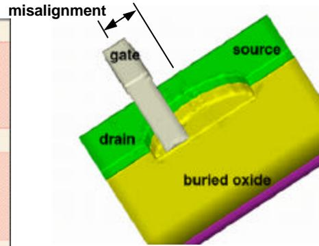
Fig.2: Half width of a 45nm narrow transistor with 25nm misalignment.
