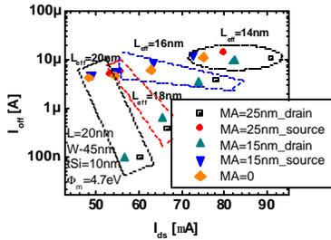
Fig.8:  $I_{on}$  and  $I_{off}$  for different misalignment and  $L_{eff}$ .
