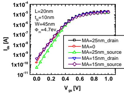
Fig.6: Simulated transfer characteristics for misaligned 45nm wide transistor ( $V_d=0.05V$ ).
