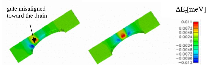
Fig.5: Change in the conduction band due to the stress in the devices with a misaligned gate (left) and with a centered gate (right). Only half width of the device is shown.
