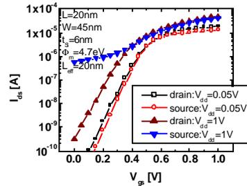
Fig.9: Transfer characteristics for narrow devices with channel thickness 6nm.
