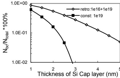
Fig. (6) The percentage of carriers in the buried channel over the total carriers at  $Q_{inv}=1e13cm^{-2}$  as a function of Si cap thickness for constant doping and retrograde doping profiles.
