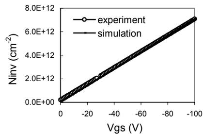
Fig. (2) Measured and simulated 2D inversion carrier density vs. gate voltage at  $V_{ds}=50mV$ .
