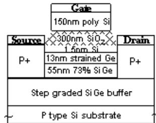
Fig. (1) Schematic cross section of the Strained-Ge buried channel PMOSFETs.
