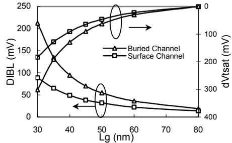
Fig. (7)  $V_{tsat}$  roll-off characteristics and DIBL of s-Ge BC PMOSFETs as compared to the Si surface channel device with a retrograde doping profile of  $1e16cm^{-3}+5e18cm^{-3}$  as shown in Fig.5.
