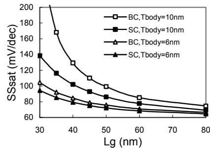
Fig. (11) Subthreshold swing vs. gate length of strained Ge BC PMOSFETs as compared to the SOI (SC) devices. A body thickness of 6nm BCGOI devices can be scaled down to 30 nm.
