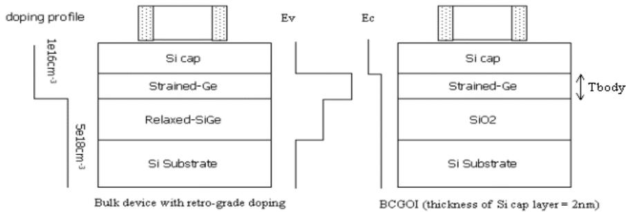
Fig. (5) Energy band offset, layer structures and retrograde doping profile of strained Ge BC PMOSFETs used in device simulation (left: bulk device with retrograde doping, right: BCGOI).
