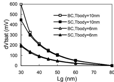
Fig. (9)  $V_{tsat}$  roll-off characteristics of s-Ge BC PMOSFETs with different channel thickness as compared to the SOI surface channel (SC) devices.
