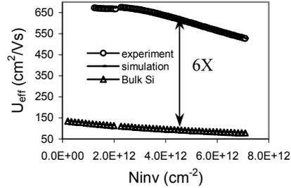
Fig. (4) Measured and simulated effective hole mobility vs. inversion charge density. Effective hole mobility of strained Ge BC PMOSFETs is more than 6X enhanced over the Si bulk universal hole mobility.
