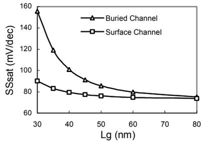
Fig. (8) Subthreshold swing vs. gate length of s-Ge BC PMOSFETs as compared to the Si surface channel device with a retrograde doping profile of  $1e16cm^{-3}+5e18cm^{-3}$ .
