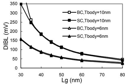
Fig. (10) DIBL of s-Ge BC PMOSFETs with different s-Ge layer thickness as compared to the SOI (SC) devices. Thinner s-Ge thickness gives better SCE control.
