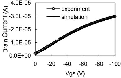
Fig. (3) Measured and simulated linear  $I_{ds}$ - $V_{gs}$  characteristics for the long channel ( $L_g=100\mu m$ ) BC PMOSFET at  $V_{ds}=50mV$ .
