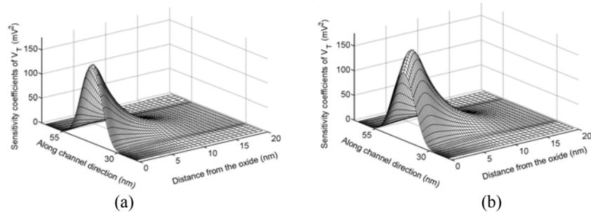
Figure 1: Sensitivity coefficients of threshold voltage for a MOSFET device: (a) classical computations and (b) quantum computations. The channel length extends from 30 nm to 55 nm in the “along channel” direction. The oxide thickness is 2 nm.
