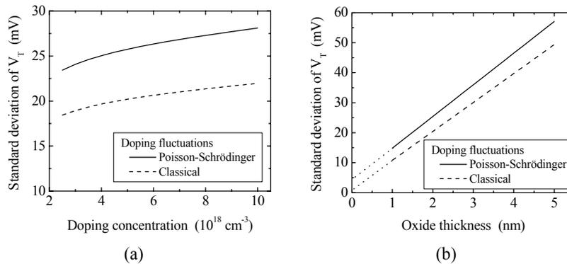
Figure 2: Standard deviation of  $V_T$  for a MOSFET device with  $L=W=25$  nm, and  $t_{ox}=2$  nm. The doping concentration indicated on the abscissa corresponds to the doping concentration at  $y=20$  nm. Only random doping induced fluctuations are considered.
