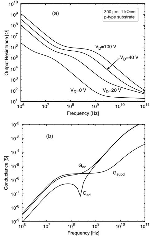
Figure 4. (a)  $R_{OUT}$  vs. frequency at different drain voltages and (b) conductance vs. frequency at  $V_D = 40$  V, made on a high resistivity 300  $\mu$ m substrate.
