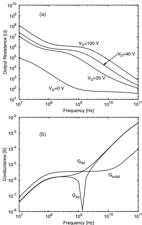
Figure 7. (a)  $R_{\text{OUT}}$  vs. frequency for different drain voltage and (b) conductance vs. frequency at  $V_D=40\text{ V}$  for the optimized substrate.
