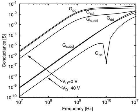
Figure 3. Conductance vs. frequency at  $V_D = 0$  and 40 V.
