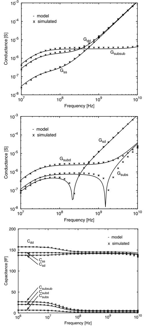
Figure 6. Modeled and simulated conductances and capacitances for the device made on a 300  $\mu\text{m}$  high resistivity substrate at  $V_D=40$  V.
