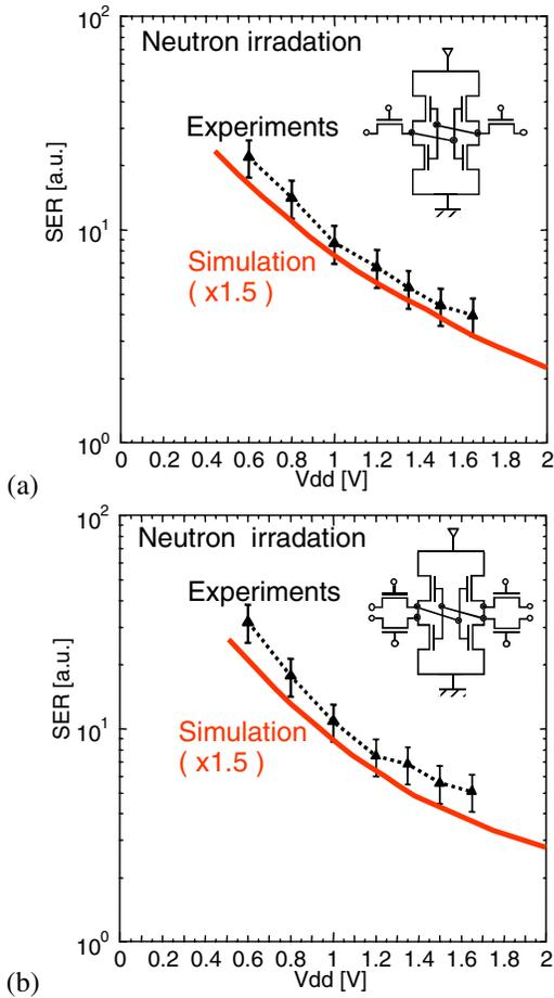
Fig. 8. Comparison between simulation results and measurement data for high-energy neutron beam acceleration tests. (a) Single-port cells, (b) dual-port cells.
