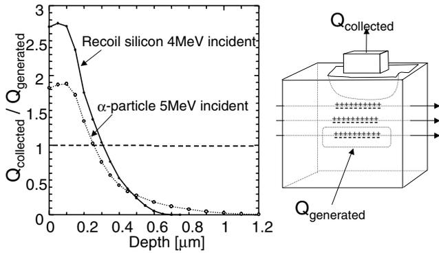
Fig. 6. Examples of the charge collection efficiency map for cases of horizontal ion penetration, calculated by a 3D transient device simulator that considered the actual doping structure of the transistors. Gain effects ( $Q_{col} > Q_{gen}$ ) can be seen for the collection charge amount at the cell nodes.
