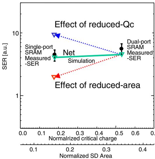
Fig. 9. Comparison between simulation (lines) and measurement (plots with error-bars) for SRAM (test-chip) cells with different configurations: single-port and dual-port. The single-port cells have about half the source/drain area and half the  $Q_c$  values, of the dual-port cells.
