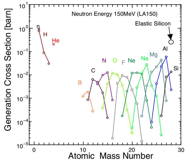
Fig. 4. Secondary ion generation cross-sections for Neutron/Silicon-nuclei reaction.
