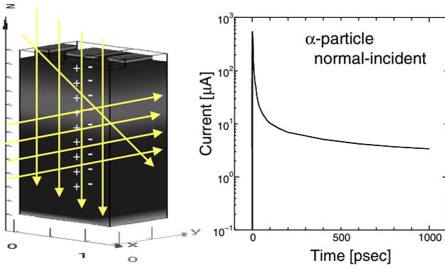
Fig. 5. 3D device simulations are performed to obtain current pulse wave forms and to construct 3D charge collection efficiency maps depending on charged particle incident positions and angles. The charge collection events are calculated based on the line charge along the ion trajectory penetrated into the unit-cells which often causes funneling effects. A typical current pulse wave form, calculated under the  $\alpha$ -particle normal incident condition, is also shown.
