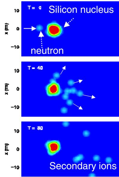
Fig. 3. Examples of QMD calculation results. About one million QMD calculations were performed combined with SDM (Statistical Decay Model) per a sampled incident neutron energy [12].
