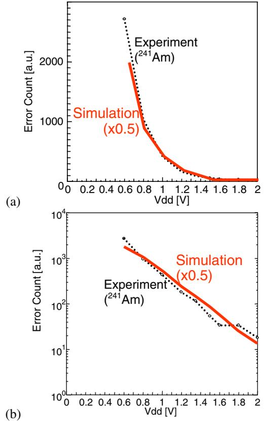
Fig. 7. Comparison between simulation and measurement for  $^{241}\text{Am}$  acceleration test. (a) Linear-scale representation, (b) log-scale representation.
