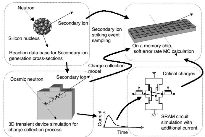
Fig. 1. SRAM soft error rate (SER) simulation system consisting of (i) nuclear-reaction database, (ii) 3D transient device simulator, (iii) circuit simulator (SPICE) and (iv) Monte Carlo SER calculation program.
