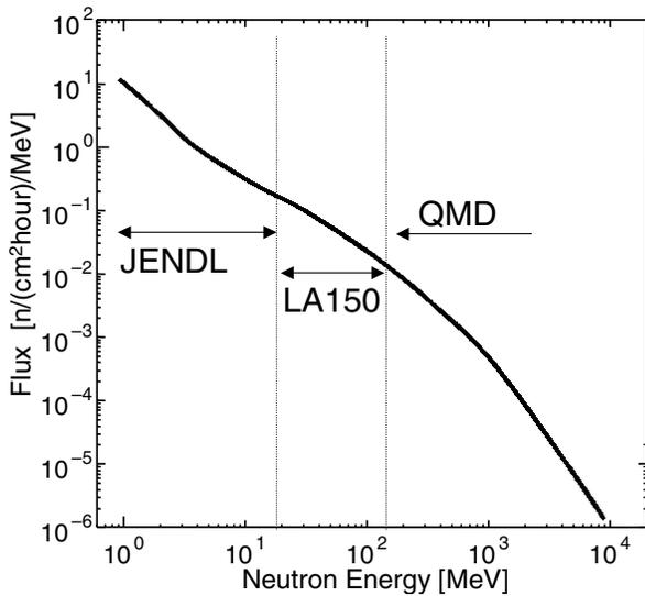
Fig. 2. Our neutron/silicon nuclear reaction data-set covering a typical cosmic-neutron energy range on earth, JENDL-3.3 for 1-20MeV [9], LA150 for 20-150MeV [10], and QMD (Quantum Molecular Dynamics) calculations for >150MeV[11]. Neutron energy flux data shown in this diagram, are taken from [14].
