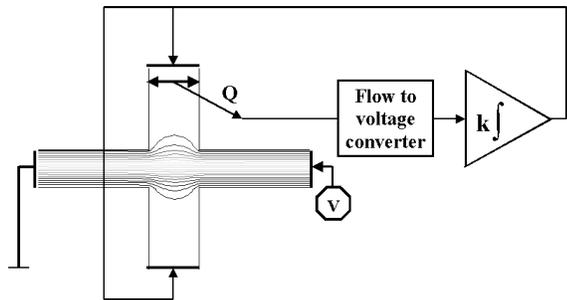
Figure 6 Block diagram of the proportional-integral control system.
