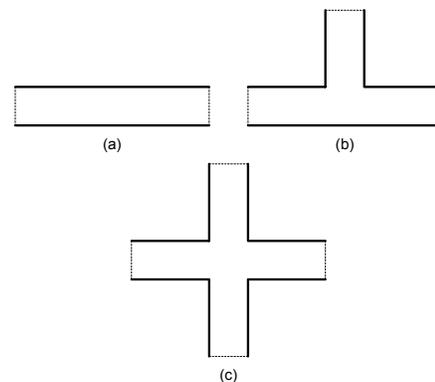
**Figure 1** Types of channels used in EOFLOW. (a) Straight channel, (b) T channel, (c) cross channel.
