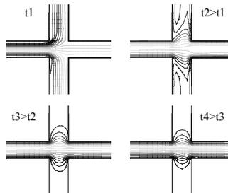
Figure 10 Dynamic behavior of streamlines for the electroosmotic system with proportional-integral control.
