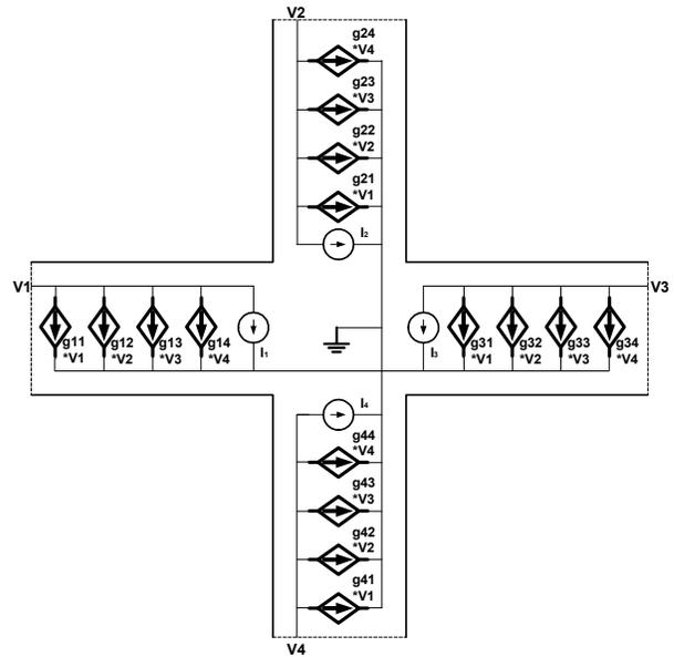
**Figure 4** SPICE3 model for cross channel.
