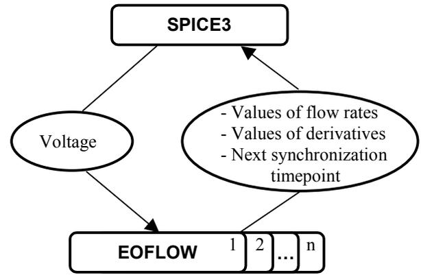
**Figure 3** Simulator block diagram.
