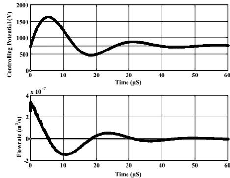
Figure 8 Dynamic behavior of controlled potentials and flow rate for the electroosmotic system with proportional-integral control.
