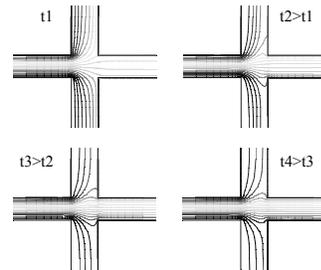
Figure 9 Dynamic behavior of streamlines for the electroosmotic system with proportional control.
