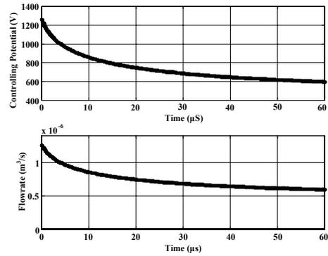
Figure 7 Dynamic behavior of controlled potentials and flow rate for the electroosmotic system with proportional control.
