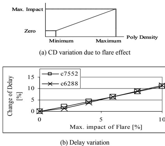
Fig. 8. Delay sensitivity to flare.
