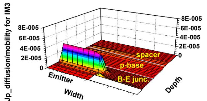
Fig.6 (c) Profile of the diffusion current density over mobility for hole of 3rd intermodulation (Carrier lifetime=1e-8sec).
