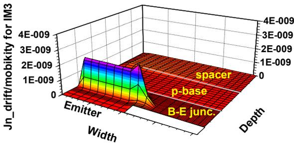
Fig.4 (b) Profile of the drift current density over mobility for electron of 3rd intermodulation (Carrier lifetime=1e-7sec).
