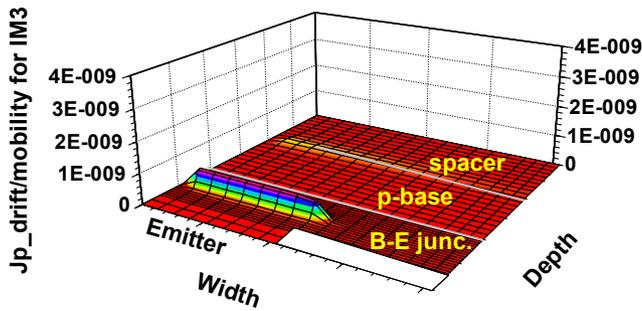
Fig.6 (a) Profile of the drift current density over mobility for hole of 3rd intermodulation (Carrier lifetime=1e-8sec).
