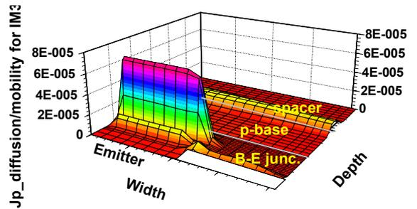
Fig.4 (c) Profile of the diffusion current density over mobility for hole of 3rd intermodulation (Carrier lifetime=1e-7sec).
