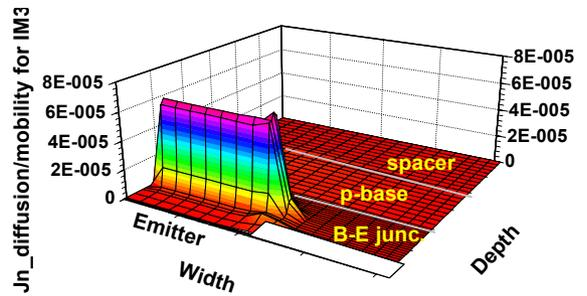
Fig.4 (d) Profile of the diffusion current density over mobility for electron of 3rd intermodulation (Carrier lifetime=1e-7sec).
