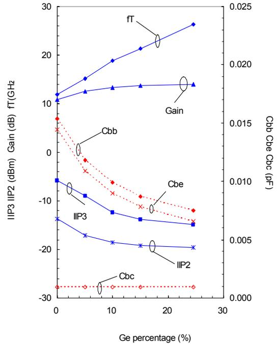
Fig.3 Ge percentage dependency of RF characteristics for the SiGe HBT with graded Ge Profile.
