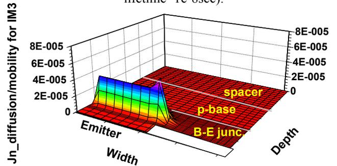
Fig.6 (d) Profile of the diffusion current density over mobility for electron of 3rd intermodulation (Carrier lifetime=1e-8sec).
