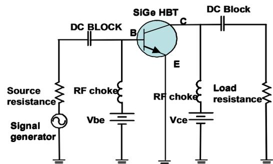
Fig.2 Circuit configuration of the mixed-mode harmonic balance device and circuit simulation of the SiGe HBT.
