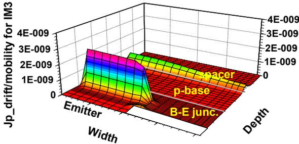
Fig.4 (a) Profile of the drift current density over mobility for hole of 3rd intermodulation (Carrier lifetime=1e-7sec).
