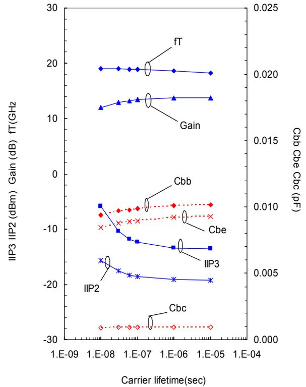
Fig.5 Carrier lifetime dependency of RF characteristics for the graded SiGe HBT with 10% Ge.
