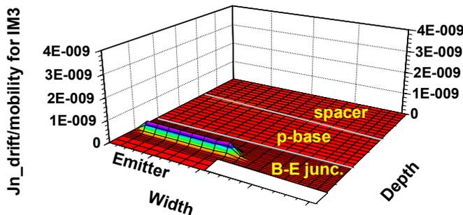
Fig.6 (b) Profile of the drift current density over mobility for electron of 3rd intermodulation (Carrier lifetime=1e-8sec).
