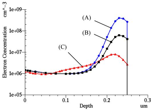
Figure 7. Simulated 1-D electron concentration at  $x=0$  (center of the channel) of each crosssection in Fig.6. With the tapered shape (C), the punch-through current near the top of the channel decreases.
