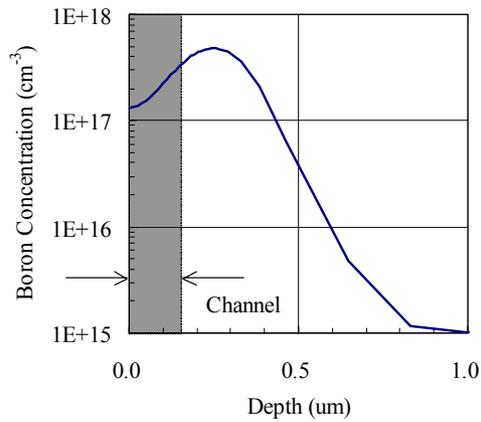
Figure 3. The optimized well profile simulated by HySyProS. The top and the bottom of the silicon pillar are located at the depth of 0μm and 0.25μm, respectively.
