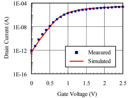
Figure 12. Measured and simulated  $I_{ds}$ - $V_{gs}$  characteristics of the fabricated device.
