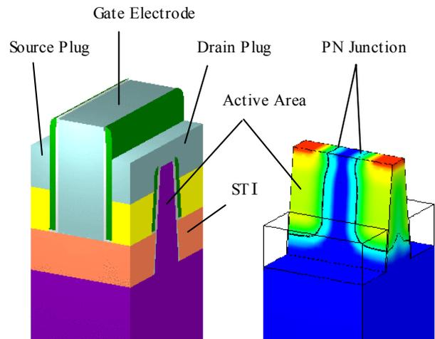
Figure 5. The device structure (left-side) and the dopant profile (right-side) simulated by HySyProS for the tapered shape (C) in Fig.4. Total number of grids is 105,748 in this case. Note that the polygonal mesh is used for incorporating the tapered-shape efficiently and accurately.
