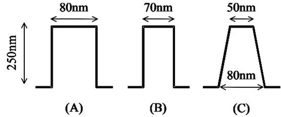
Figure 4. A schematic illustration of a cross-section of the silicon pillar. Two ideal block-shaped pillars with different thicknesses (A) (B) and a taper-shaped pillar (C) are examined. The initially estimated shape is (A), meanwhile, the actual shape of the fabricated device is (C).
