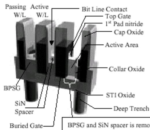
Figure 1. A schematic of the target DRAM device. It includes two unit cells that share the bit-line contact. The FinFET consists of the pillar-shaped active area and the fin-shaped buried gate, which operates as a transfer gate.
