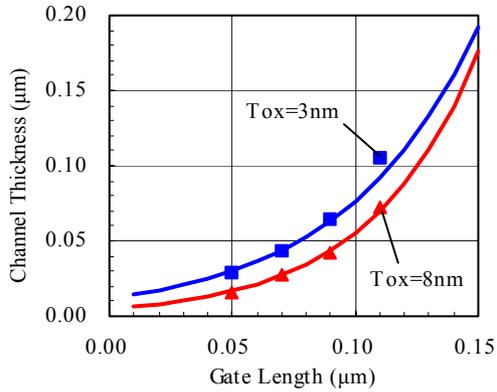
Figure 2. The channel thickness required for the off-leak current of 0.1fA. The square and the triangular symbols represent simulated results for the gate oxide thickness of 3nm and 8nm, respectively.
