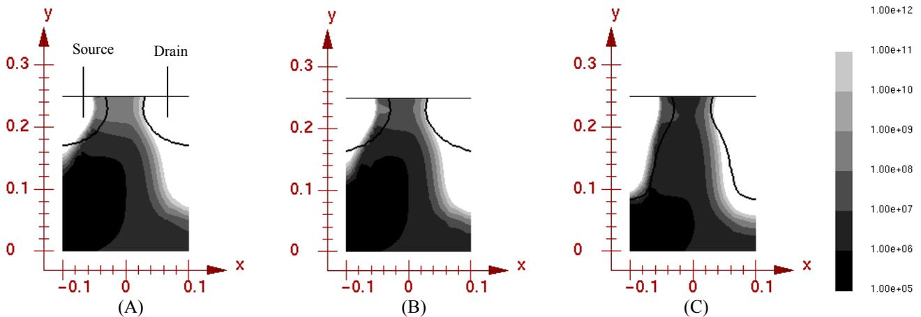
Figure 6. Simulated 2-D electron concentration at the off state on a cross-section at the middle of the silicon pillar for each shape in Fig.4. The solid lines in the source and drain regions indicate the metallurgical PN-junctions.
