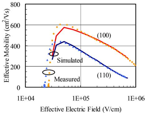
Figure 9. Measured (marks) and simulated (lines) universal curves for (100) and (110) crystalline planes at the temperature of 347K.
