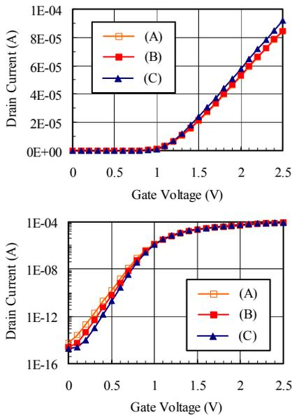
Figure 8. Simulated  $I_{ds}$ - $V_{gs}$  characteristics for the three different shapes of the silicon pillars in Fig.4. The tapered-shape (C) gives higher drive current and lower off-leak current than others.
