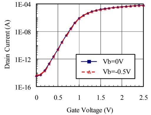
Figure 11. Simulated  $I_{ds}$ - $V_{gs}$  characteristics after the optimization of the dopant profiles. The contact resistances of the source and drain plugs are included in the simulation.
