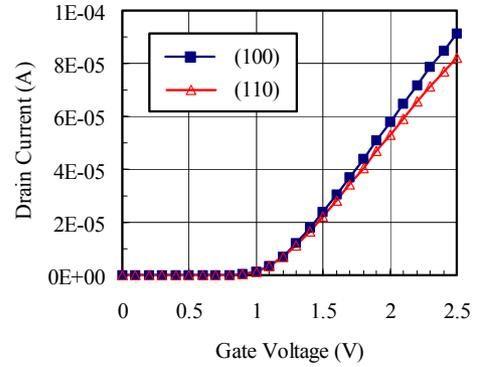
Figure 10. Simulated  $I_{ds}$ - $V_{gs}$  characteristics with (100) and (110) mobility models.
