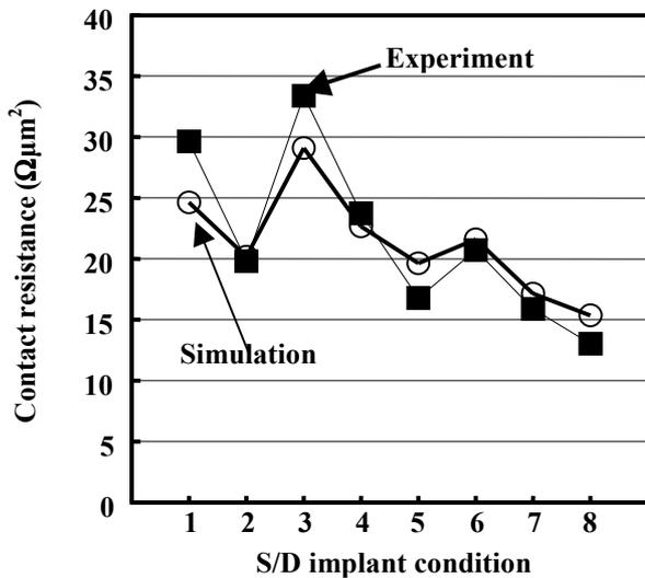
Figure 7. The contact resistance for NiSi/ n<sup>+</sup>Si. Open circles are simulation results, solid squares are experimental data.
