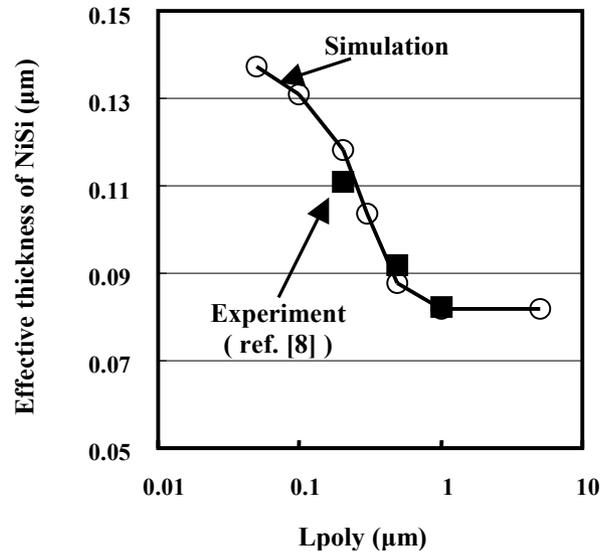
Figure 5. Effective thickness of NiSi versus gate polysilicon length. Open circles are simulation results, solid squares are experimental data [8].
