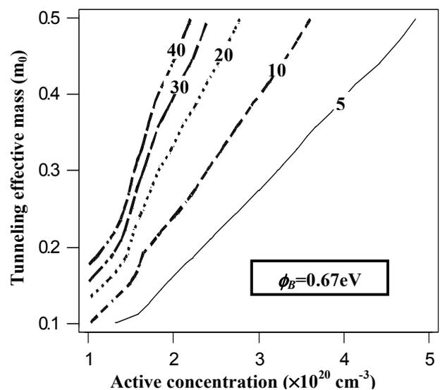
Figure 6. Contour plot for the contact resistance in  $n^+\text{Si}$ . The unit of the contact resistance is  $\Omega\mu\text{m}^2$ .
