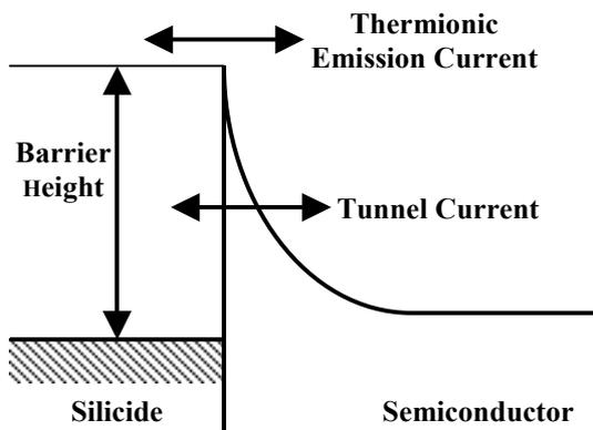
Figure 2. Schematic band diagram at the interface between silicide and semiconductor.
