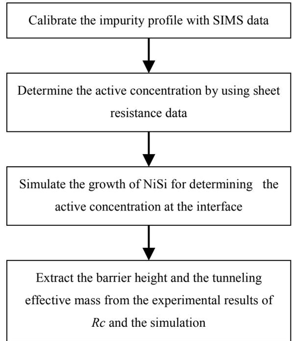
Figure 3. Calibration strategy of the contact resistance at the interface between NiSi and silicon substrate.
