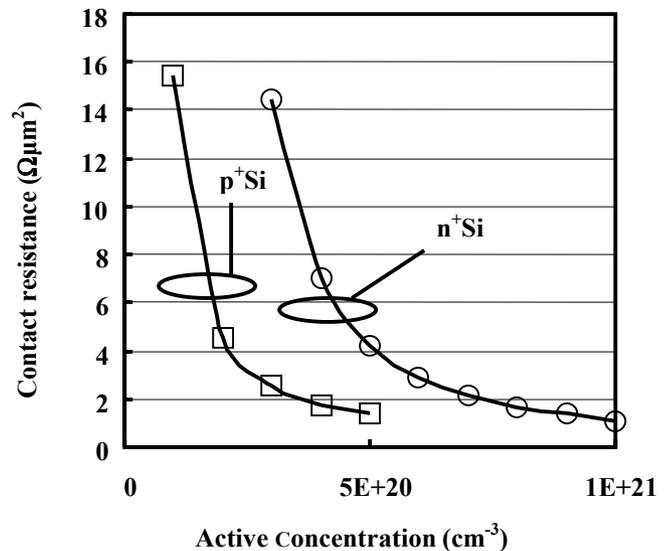
Figure 9. Simulation results of the contact resistance for active concentration at the NiSi/ Si interface.
