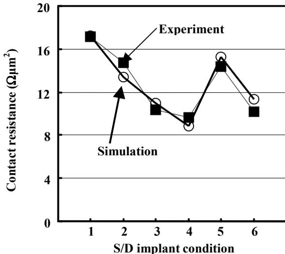
Figure 8. The contact resistance for NiSi/ p<sup>+</sup>Si. Open circles are simulation results, solid squares are experimental data.
