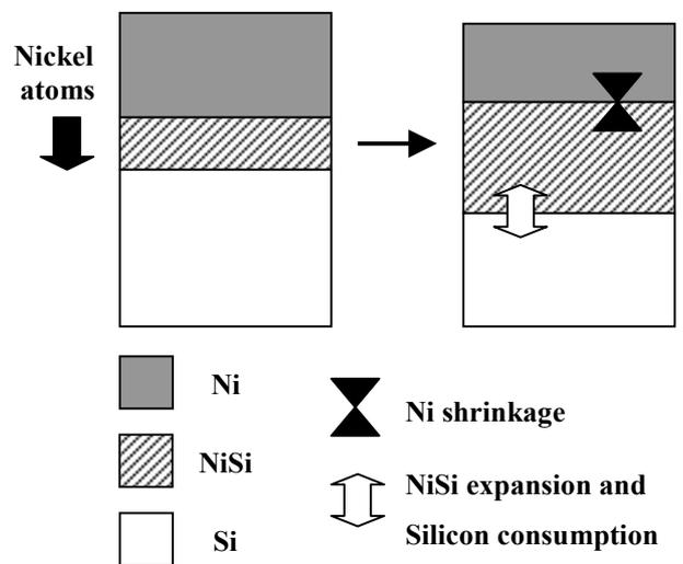
Figure 1. Schematic illustration of the growth mechanism during nickel silicidation.
