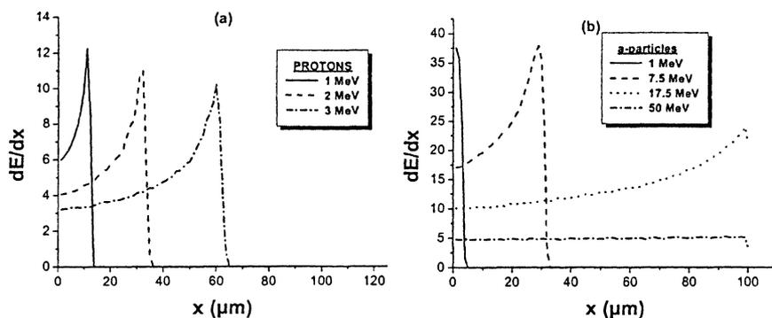
**Fig. 1.** Bragg curves indicating the energy deposition of (a) protons in a 125 $\mu\text{m}$  thick bulk GaAs detector, (b)  $\alpha$ -particles in a 100 $\mu\text{m}$  thick bulk GaAs detector. The ionization of the detector is proportional to the particle's energy loss  $dE/dx$ .
