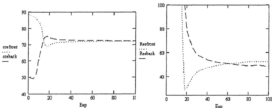
**Fig. 2.** Energy dependence of the c.c.e (left) and energy resolution (right) calculated for a bulk SI GaAs 100 $\mu\text{m}$  thick detector irradiated by  $\alpha$ -particles with energy range 1–100 MeV.
