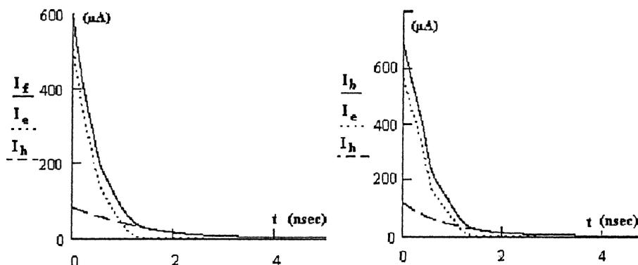
**Fig. 4.** Simulated current pulse during the 17.5 MeV front (left) and back (right) irradiation of a 100 $\mu\text{m}$  thick bulk GaAs detector operating in pulse mode. The electron (dot) and hole (dash) current components resultant is the total current (solid).
