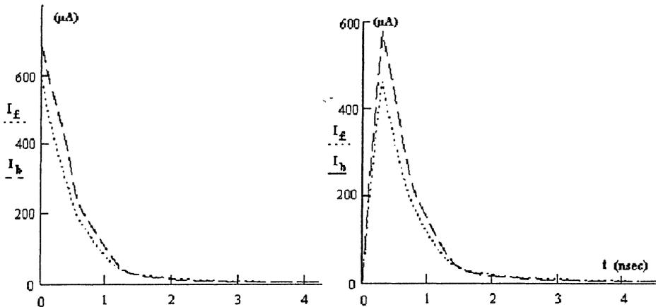
**Fig. 3.** Calculated current pulse produced by a GaAs detector when irradiated from the Schottky contact (dotted) or the ohmic contact (dashed) when operating in pulse mode (left) and current mode (right).
