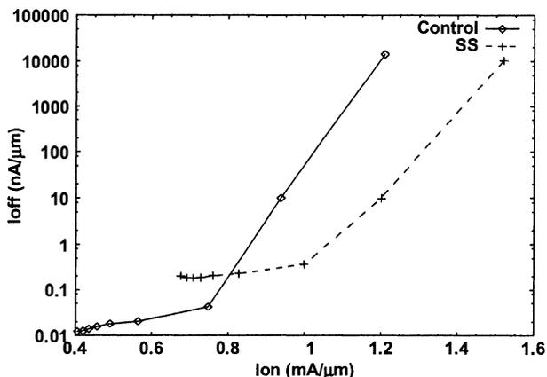
Fig. 4.  $I_{on}/I_{off}$  characteristics of the control and strained silicon devices. Significantly higher on currents can be obtained using strained silicon. Off currents for long channel length strained silicon devices are larger than the control devices due to higher junction leakage.
