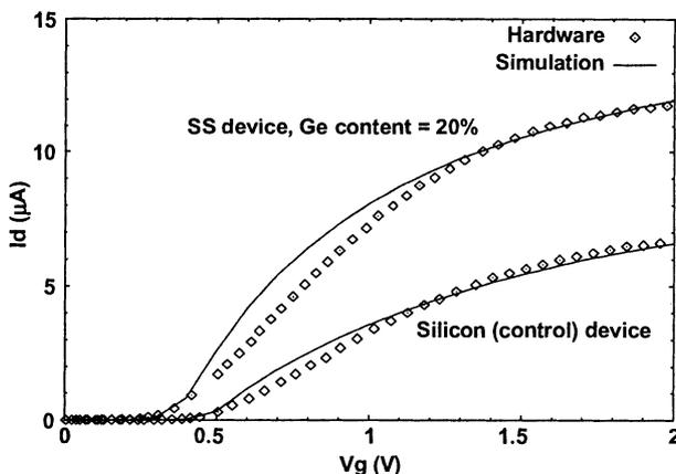
Fig. 1. Comparison of measured and simulated linear  $I_d$ - $V_g$  characteristics of 10X10 strained and unstrained silicon devices.
