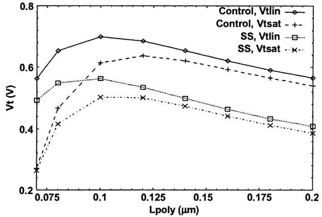
Fig. 2.  $V_t$  roll off characteristics of the control and strained silicon devices.  $V_{\text{tsat}}$  for the 70 nm gate length devices are similar due to the constraint of off current being  $10 \text{ nA}/\mu\text{m}$ .
