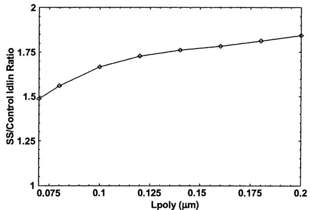
Fig. 3. Ratio of linear current for strained silicon and control devices as a function of gate length.
