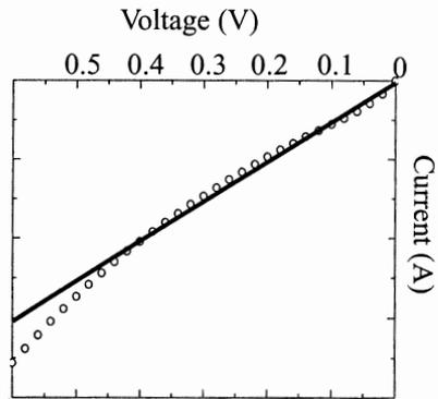
Fig.5. The reverse current characteristic of diode and nominal conductance.
