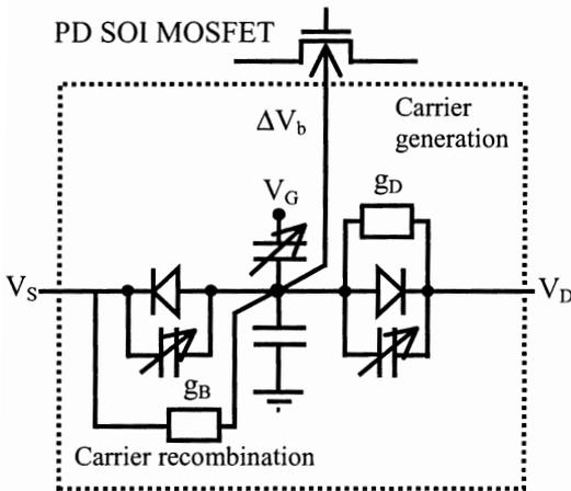
Fig.4. Dashed rectangle: a sub-circuit to track transient behavior of floating body potential,  $\Delta V_b$ , which controls the threshold voltage of PD SOI MOSFET.
