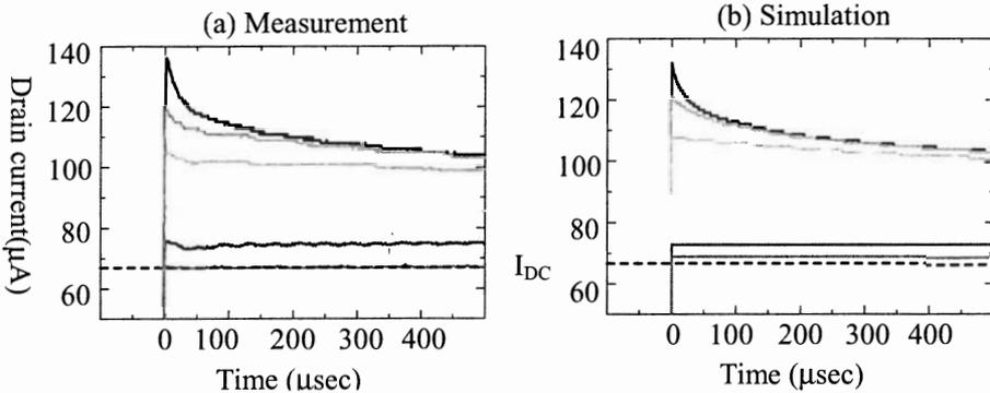
Fig.2. Transient drain current as a parameter “off” duration:  $t_{off}=10\mu$ sec(bottom) to 100msec(top).  $I_{DC}$  represents the steady state drain current at DC bias condition.
