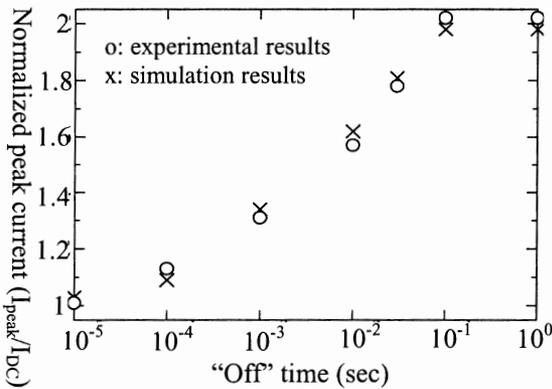
Fig.6. Normalized peak current as a function of "off" duration. Open circles: measured results and Crossed are simulated results
