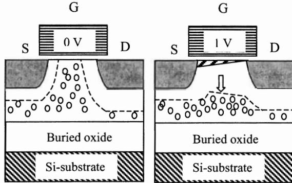
Fig.3. At “switch on”, holes near the surface are squeezed into the floating body, leading to positive charged body.
