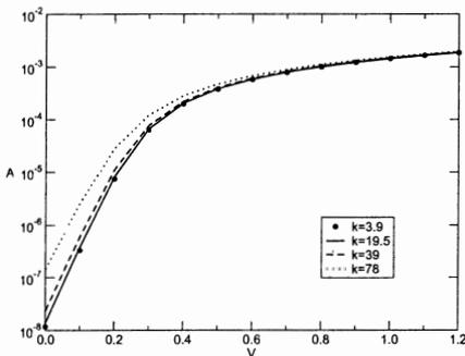
Fig. 4: Transfer Characteristics
