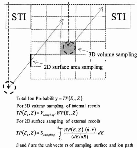
**Fig. 5.** The novel technique for effective sampling of recoil ions initiated inside and outside the charge collection box underneath S/D area. The surface area sampling comprehends all recoil ions initiated outside but eventually entering the box.
