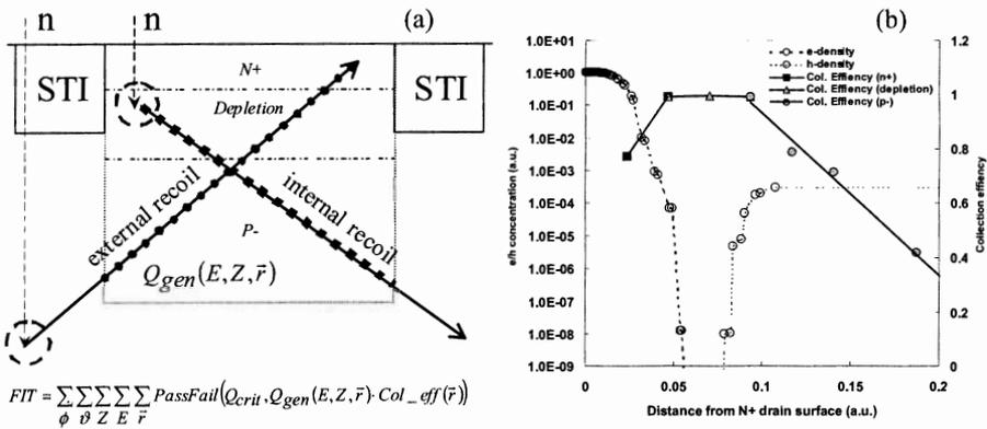
Fig. 4 (a) Charge generation model and the general equation for charge collection and FIT calculation; (b) Charge collection efficiency derived from 3D device simulations and its correspondence to the S/D-to-well junction doping profile
