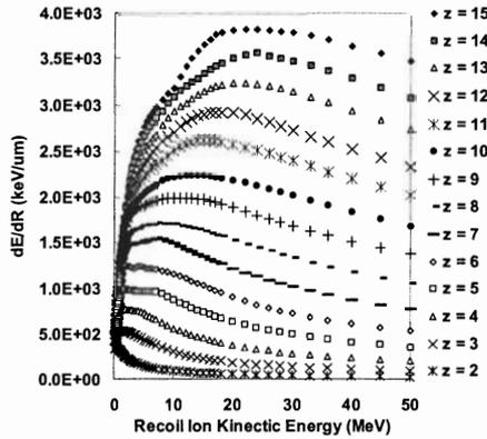
Fig. 3. Recoil ion energy loss rate in silicon, simulated using TRIM [13]
