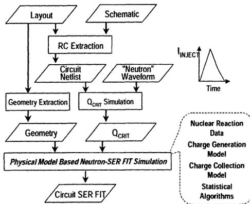
Fig. 1. Neutron-SER modeling and simulation methodology and flow
