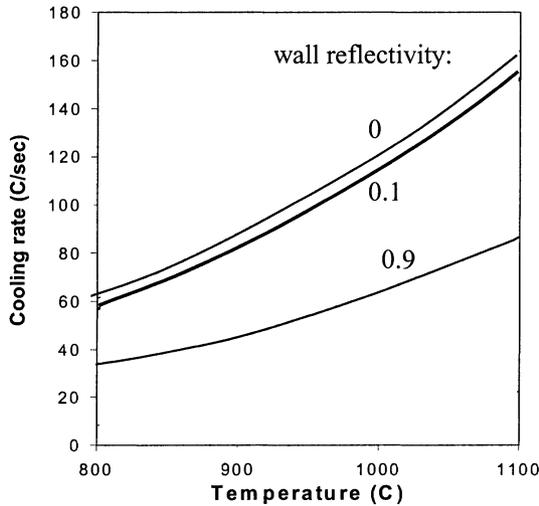
**Figure 2:** Cooling rate versus temperature for three values of  $r$ , with  $a=0.2$ , representing the effect of a quartz window between the wafer and the wall.
