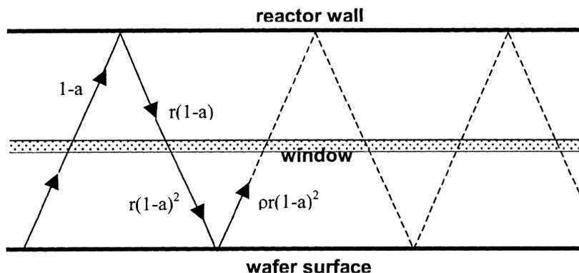
**Figure 1:** Schematic of radiation transport in the RTP reactor.
