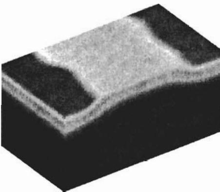
**Fig. 7.** Potential distribution at threshold in a well scaled 30×30 nm MOSFET with line edge roughness of the gate of 6 nm.
