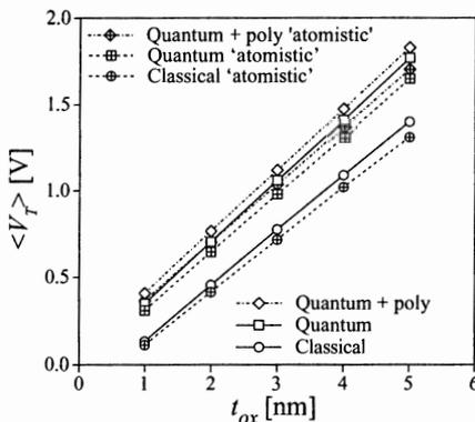
**Fig. 3.** Dependence of average threshold voltage on the gate oxide thickness in a  $50 \times 50$  nm MOSFET.
