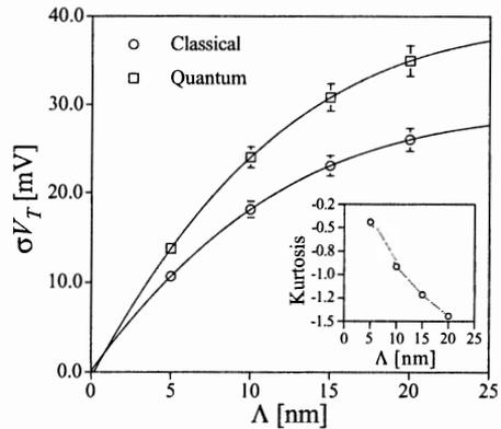
**Fig. 6.** Dependence of the threshold voltage standard deviation  $\sigma V_T$  on the correlation length  $\Lambda$  for the 30×30 nm MOSFETs as in Fig. 5. Classical and DG simulation results are compared.
