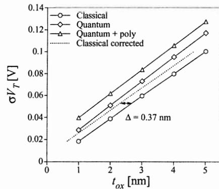
**Fig. 4.** Threshold voltage standard deviation as a function of the oxide thickness in a  $50 \times 50$  nm MOSFET.
