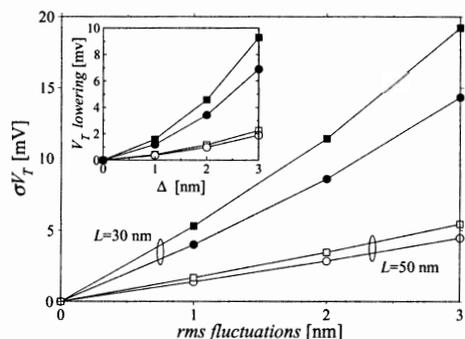
**Fig. 8.** Threshold voltage fluctuations associated with LER as a function of the rms amplitude  $\Delta$ .
