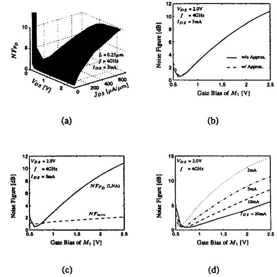
Fig. 5. Power constrained noise figure ( $N_{F_{PD}}$  [dB]) of the tuned amplifier when  $R_s = Z_{in} = 50\Omega$ ,  $L = 0.25\mu m$ , and the current is fixed to 5mA. (a) For the entire operating range. (b) Comparison to the approximation. The solid line is the actual noise figure; the dashed line is the approximated results using (23). (c) Comparison to the intrinsic  $N_{F_{min}}$  of the MOSFET. (d)  $N_{F_{PD}}$  for different current specifications.
