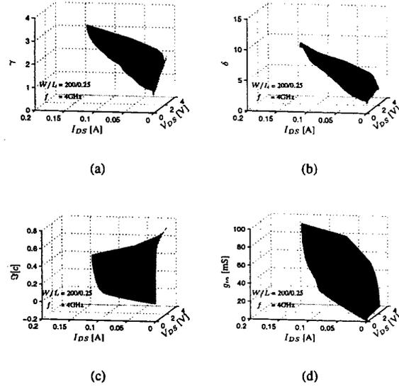
Fig. 1. Intrinsic noise parameters for the entire operating range of 0.25  $\mu\text{m}$  nMOSFET. (a) Drain noise parameter ( $\gamma$ ). (b) Gate noise parameter ( $\delta$ ). (c) Cross correlation between the drain and the gate noise (the imaginary part of c). (d) Transconductance ( $g_m$ ).
