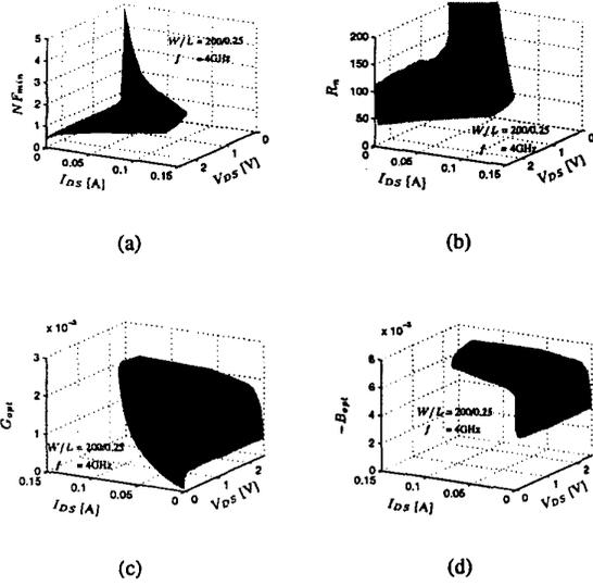
Fig. 2. Intrinsic noise performance for the entire operating range of a 0.25  $\mu\text{m}$  nMOSFET. (a) Minimum noise figure ( $NF_{min}$  [dB]). (b) Equivalent noise resistance ( $R_n$  [ $\Omega$ ]). (c) Optimum source conductance ( $G_{opt}$  [S]). (d) Optimum source susceptance ( $B_{opt}$  [S]).
