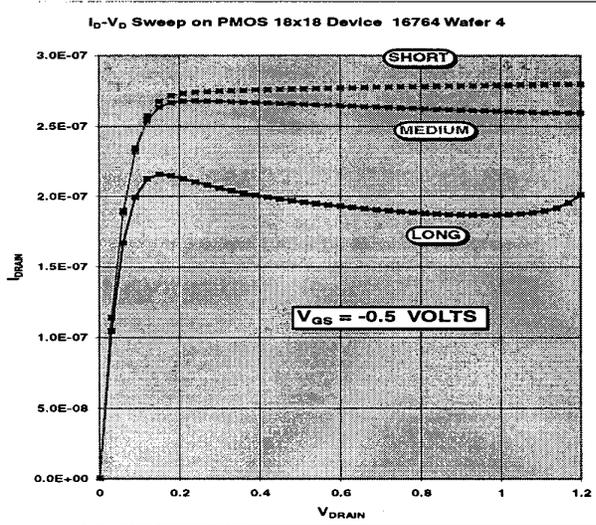
Fig. 4: Experimental data of a 10  $\mu\text{m}$  PMOS device employing various integration times of the HP4156.
