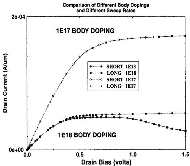
Fig. 5: Transient  $I_D-V_D$  sweep for constant body doping of  $10^{17}$  and  $10^{18}$ . LONG corresponds to 20 seconds from 0 to 1.5 volts, and SHORT corresponds to 1 millisecond from 0 to 1.5. Note the loss of any difference between the sweeps for the  $10^{17}$  case.
