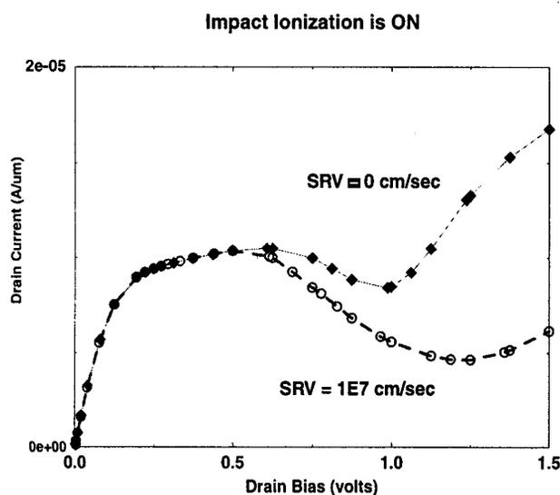
Fig. 7:  $I_D$ - $V_D$  curve for a buried-oxide surface recombination velocity (SRV) of 0 and  $10^7$  cm/sec.
