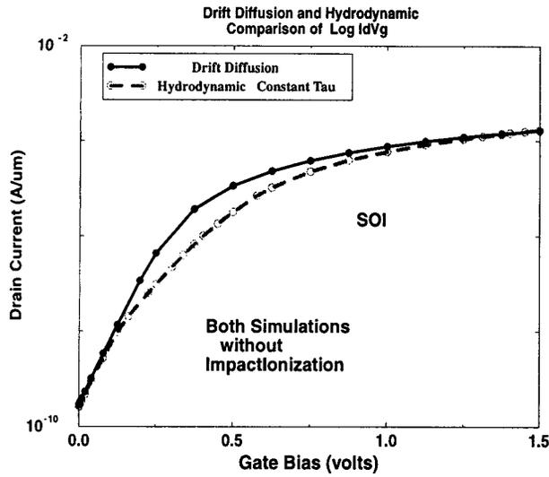
Fig. 1: 1  $\mu\text{m}$  device. Drift-Diffusion (DD) and HydroDynamic (HD) (both without impact-ionization)  $\log I_D-V_G$  comparison. Constant energy relaxation time of 0.3 ps.  $V_{DS} = 1.5$  volts. The HD simulation shows a change in body potential from hot-carrier diffusion out of the channel, resulting in a decrease in drain current.
