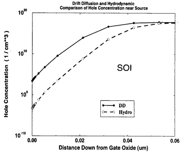
Fig. 2: Hole concentration near source for  $V_{GS} = 0.375$  from Fig. 1. Note the differing depletion regions.
