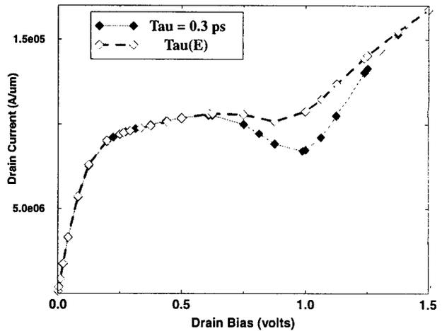
Fig. 3: HD (WITH impact-ionization)  $I_D-V_D$  sweep with a constant, and an energy-dependent relaxation time. The latter results in lower carrier temperatures and less diffusion of the hot carriers into the body.
