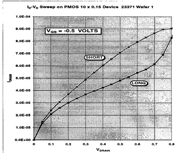
Fig. 6: PMOS device with gate length of approximately 0.15  $\mu\text{m}$  from a later lot, which possessed lower well doping, but an increased halo dose, resulting in approximately the same body doping for the long PMOS device of Fig. 4.
