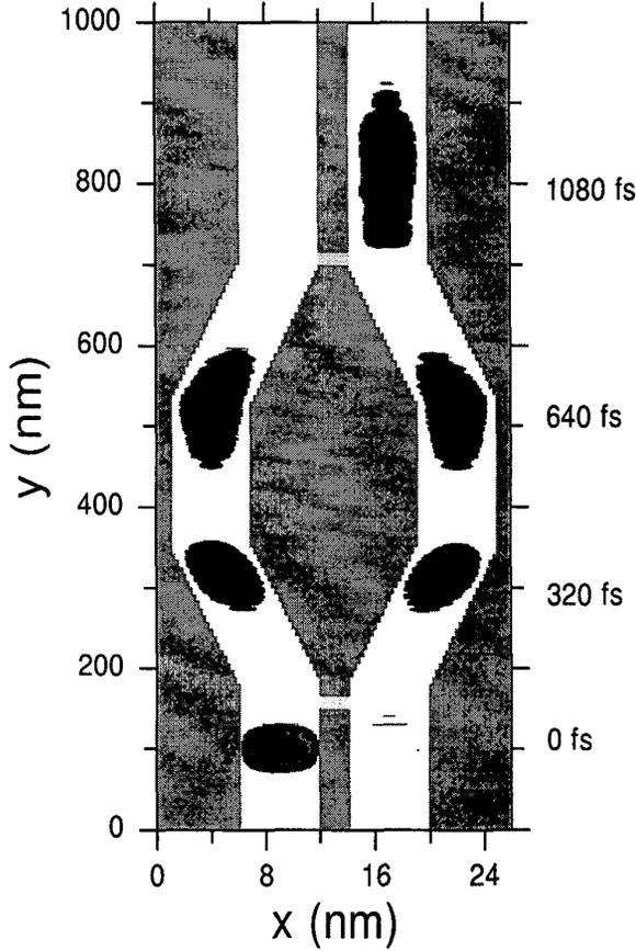
Fig. 1. Electron density at different times in the proposed device: two coupling windows between the wires are applied, which realize the “beam splitter” gate. A quantum NOT is obtained.
