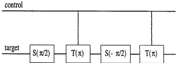
Fig. 4. A network consisting of two  $\mathbf{T}(\phi)$  gates and two  $\mathbf{S}(\theta)$  gates can simulate the C-NOT.
