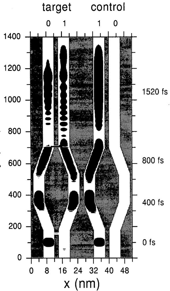
Fig. 6. Electron density at different times in the device corresponding to Eq. (7). The control qubit is  $|1\rangle$ , hence the Coulomb interaction between the electrons delays the wave functions propagating in the inner wires. The initial state  $|10\rangle$  is evolved to the final state  $(1 - i)(|10\rangle - |11\rangle)/2$ .
