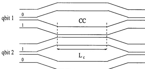
Fig. 3. Architecture for the  $\mathbf{T}(\phi)$  gate based on the Coulomb coupler CC: the phase  $\phi$  is proportional to the coupler length  $L_c$ .
