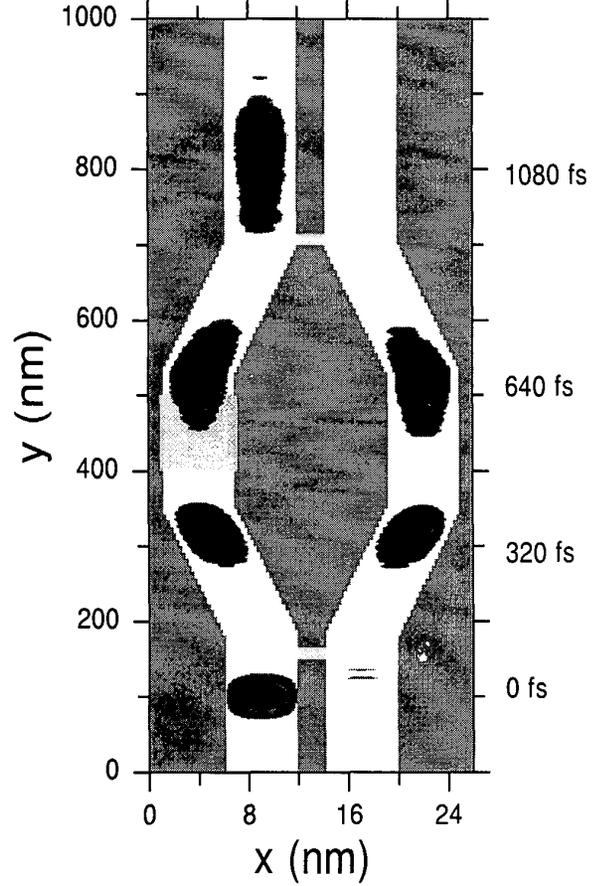
Fig. 2. Electron density at different times in the proposed device: two “beam splitter” gates are applied with a delaying potential between them in one of the wires (light grey region). A quantum IDENTITY is obtained.
