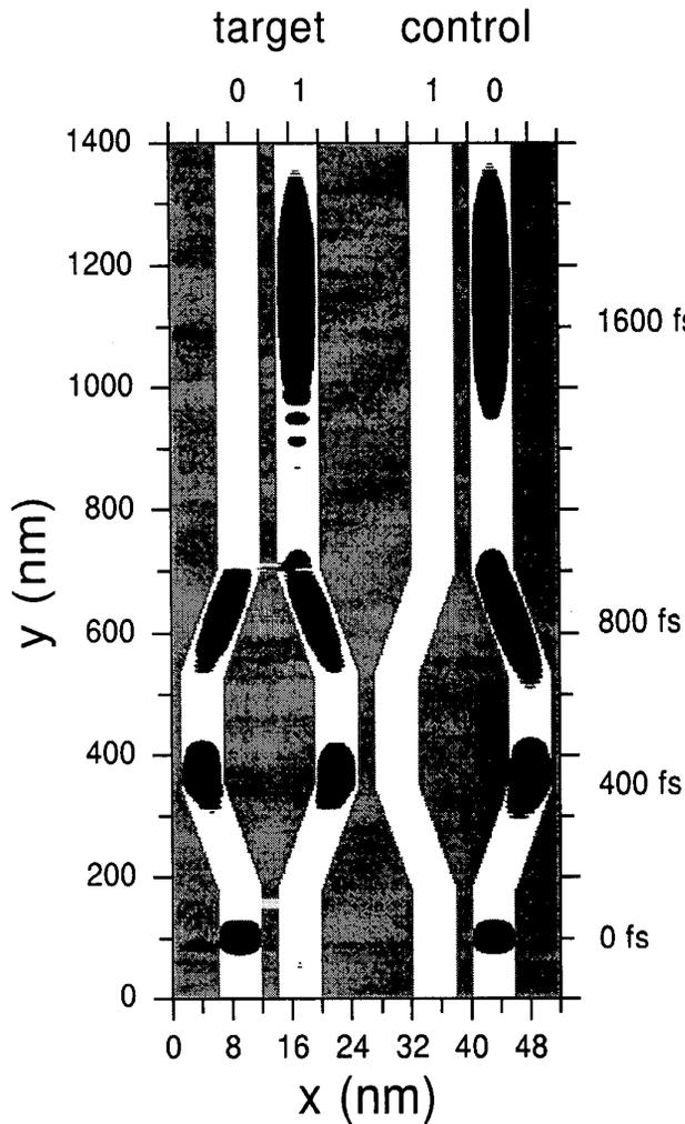
Fig. 5. Electron density at different times in the device corresponding to Eq. (7). As the control qubit is  $|0\rangle$ , the Coulomb interaction between the electrons is not effective due to the large distance. The initial state  $|00\rangle$  evolves to the final state  $|01\rangle$ , due to the action of the two beam splitters applied to the target qubit.
