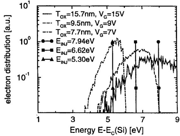
Fig. 5. Electron distributions at the oxide-silicon interface for  $T_{OX} = 15.7$  nm,  $V_G = 15$  V (solid),  $T_{OX} = 9.5$  nm,  $V_G = 9$  V (dashed),  $T_{OX} = 7.7$  nm,  $V_G = 7$  V (dot-dashed). The corresponding average energies  $E_{inj}$  are marked by vertical lines.
