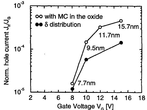
Fig. 8. Ratio between the hole current injected back in the oxide ( $J_h$ ) and the corresponding electron current  $J_G$  in MOS capacitors featuring  $T_{ox} = 7.7, 9.5, 11.7$  and  $15.7$  nm.
