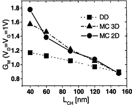
Fig. 5: transconductance S/mm for devices of fig. 4.
