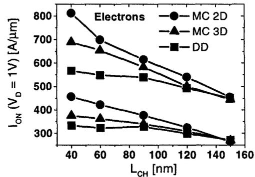
Fig. 4: nMOS  $I_{ON}$  as a function of  $L_{CH}$  with  $\mu_0 = 300 \text{ cm}^2 / \text{Vs}$  and  $V_{GS}=0.8\text{V}$  and  $1\text{V}$ .
