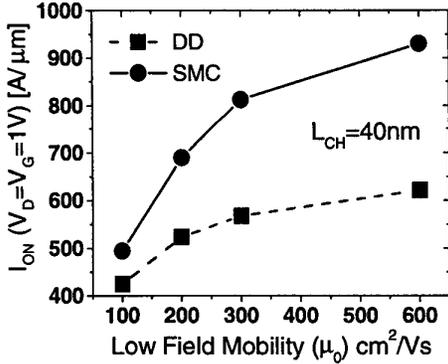
Fig. 6:  $I_{ON}$  as a function of  $\mu_0$  for a  $L_{CH} = 40\text{nm}$  nMOSFET.
