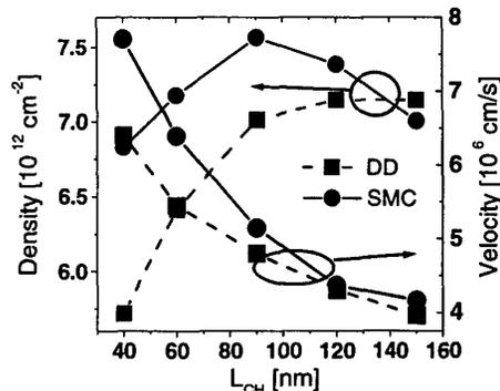
Fig. 3:  $n_{IN}$  and  $v_{IN}$  at the top of the source barrier as a function of  $L_{CH}$  with  $V_{GS}=V_{DS}=1\text{V}$ . Averages as in fig. 3.  $\mu_0 = 300 \text{ cm}^2 / \text{Vs}$ . Note,  $I_D = q n_{IN} v_{IN}$ .
