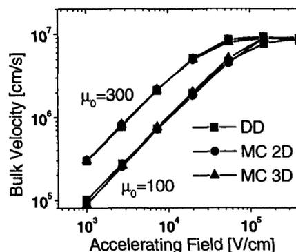
Fig. 1: Comparison of electron field dependent velocity (constant field) with  $\mu_0=300\text{cm}^2/\text{Vs}$  and  $100\text{cm}^2/\text{Vs}$ .
