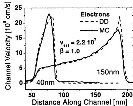
Fig. 8: Channel velocity for electrons (see fig. 2) with  $\beta=1$ ,  $v_{sat}=2.2 \times 10^7$   $\text{cm}/\text{s}$  in the DD model.
