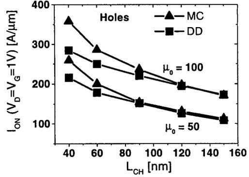
Fig. 7: pMOS  $I_{ON}$  as a function of  $L_{CH}$  for  $V_G=V_D=1\text{V}$  with  $\mu_0 = 100$  and  $50\text{cm}^2/\text{Vs}$ .
