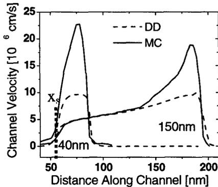
Fig. 2: Channel velocity in  $L_{CH} = 40\text{nm}$  and  $150\text{nm}$  devices averaged perpendicularly from the oxide interface through  $4\text{nm}$  of the channel.
