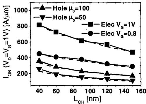
Fig. 9:  $I_{ON}$  for nMOS and pMOS with  $V_D=1V$ . Dashed lines: DD using  $\beta=1$ ,  $v_{sat}=2.2 \cdot 10^7$  cm/s for electrons,  $\beta=0.65$ ,  $v_{sat}=1.5 \cdot 10^7$  cm/s for holes; solid lines are MC. For electrons,  $\mu_0=300$  cm<sup>2</sup>/Vs; for holes  $V_G=1V$ .
