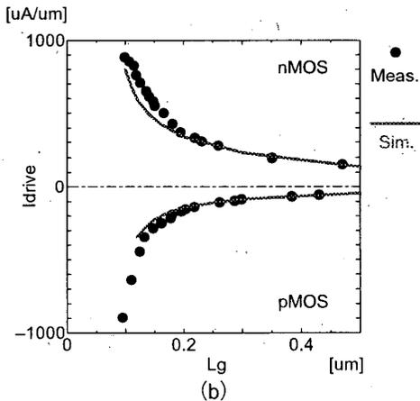
Fig. 7 Comparison of the (a)  $V_t$ - $L_g$  and the (b)  $I_{drive}$ - $L_g$  characteristics between the measurement and the simulation for the CMOS fabricated without pocket I/I.  $V_t$  shows reasonable agreement. Even a drift-diffusion type device simulator can predict  $I_{drive}$  with good accuracy.
