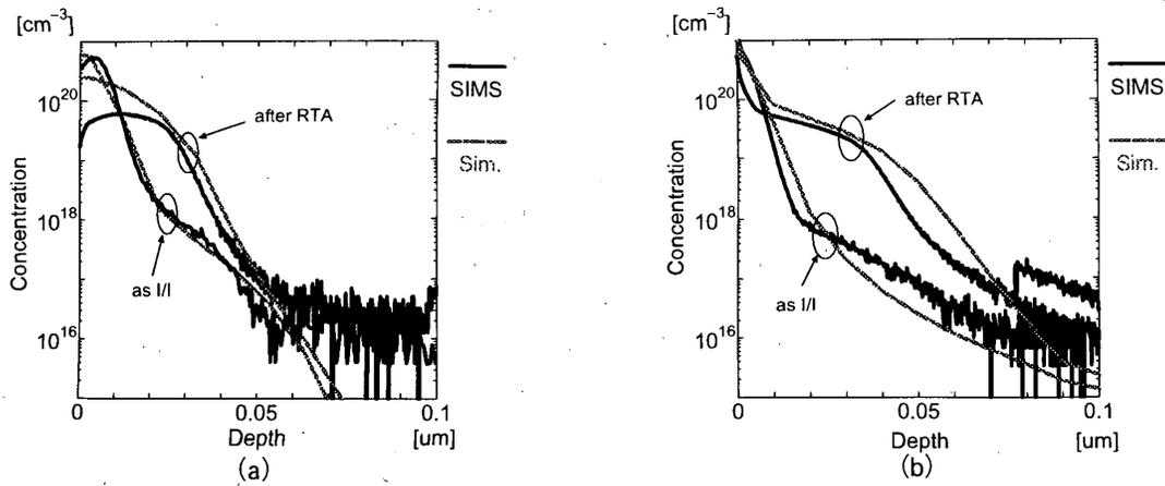
Fig.1 B, P, As and point-defect pair diffusion model with a unified parameter set can reproduce the ultra shallow S/D-extension profiles except for the out-diffusion from the surface. (a)As for nMOS. (b) B for pMOS.
