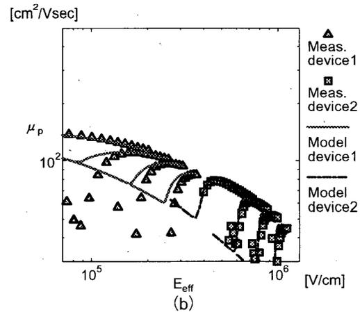
Fig.3 MOS surface mobility model including the vertical field dependent Coulomb screening effect can reproduce the measurement both in the roll-off and the universality regions. (a) electron mobility. (b) hole mobility.
