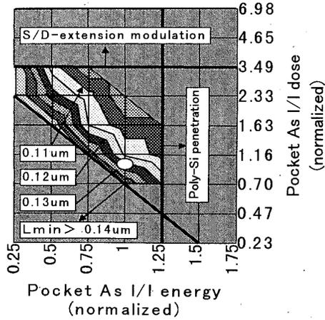
Fig. 5 Lmin vs pMOS tilted pocket As I/I condition map. The circle is an adopted design point.
