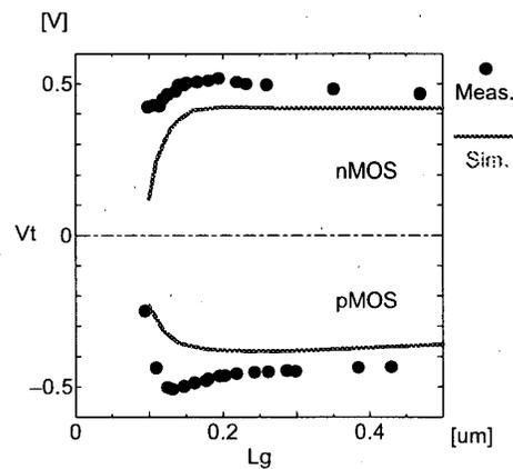
Fig. 8 Comparison of the  $V_t$ - $L_g$  characteristics for the CMOS with pocket I/I. Further model improvement is required for more accurate prediction.
