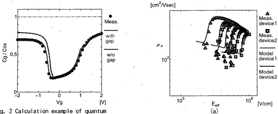
Fig. 2 Calculation example of quantum mechanical model. By inserting the low concentration thin gap layer at the interface between poly-Si and gate oxide, the measured full Cg-Vg characteristics can be reproduced.
