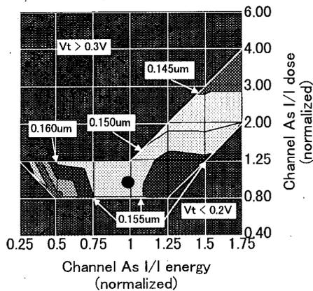
Fig. 4 Lmin vs pMOS channel As I/I condition map calculated by using TCAD. The circle is an adopted design point.
