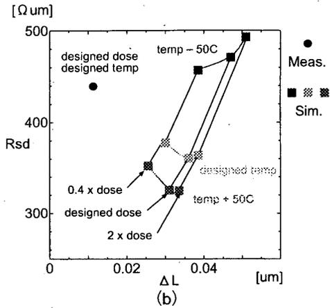
Fig. 6 Comparison of the  $\Delta L$ - $R_{sd}$  characteristics between the measurement and the simulation. (a) The simulation shows a reasonable predictability for nMOS. (b) The simulation overestimates  $\Delta L$  in pMOS.
