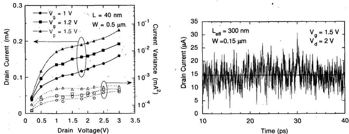
Figure 1: (a) Typical drain voltage dependence of the drain current (left scale) and the variance of the drain current (right scale)  $\langle \delta I^2 \rangle$ , obtained from the MC simulations for the n-channel Si-MOSFET with  $L_{\text{eff}} = 40$  nm and  $W = 500$  nm. (b) Time series of the drain current in the n-channel Si-MOSFET with  $L_{\text{eff}} = 300$  nm and  $W = 150$  nm.
