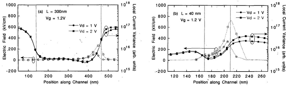
Figure 3: Local current variances  $\sigma_{loc}^2$  as a function of the position along the channel for Si-MOSFETs with (a)  $L_{eff} = 40$  nm and (b)  $L_{eff} = 300$  nm.
