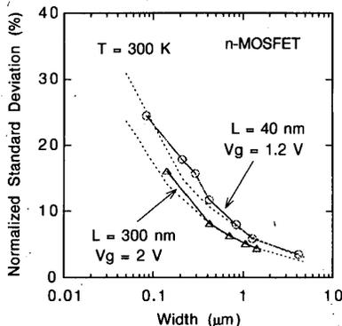
Figure 2: Normalized standard deviation of the drain current:  $\langle \delta I^2 \rangle / I_{ave}$  as a function of the device width  $W$  of Si-MOSFETs with the channel length of  $L_{eff} = 40$  and  $300$  nm. The dotted line is the prediction described in the text;  $\langle \delta I^2 \rangle / I_{ave} \propto W^{-1/2}$ .
