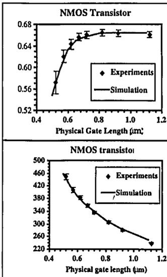
**Figure 1** Comparison between simulation and experiments,  $V_t$  (top) and saturation current (bottom) for the NMOS transistor. The physical gate length is the one drawn with  $0.05\mu\text{m}$  bias per side.
