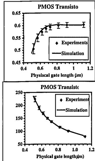
**Figure 2** Comparison between simulation and experiments,  $V_t$  (top) and saturation current (bottom) for the PMOS transistor. The physical gate length is the one drawn with  $0.05\mu\text{m}$  bias per side.
