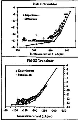
**Figure 3** Comparison between simulation and experiments for the leakage current ( $V_{DS}=3.63V$ ) vs. saturation current ( $V_{DS}=V_{GS}=3.3V$ ) for NMOS (top) and PMOS (bottom).
